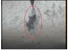
(e) After 4h of tree initiation Fig. 7. Electrical tree growth pattern in epoxy-silica nanocomposite. Tree growth can be seen inside the circle
