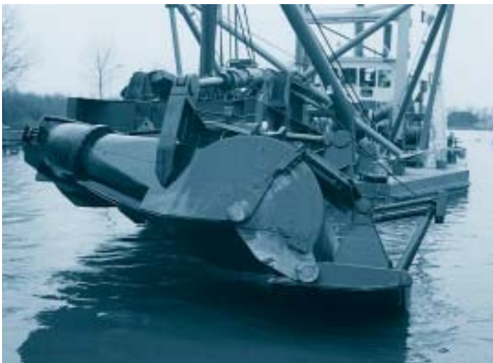
Figure 2. Close up of a specially developed environmental sweephead.
