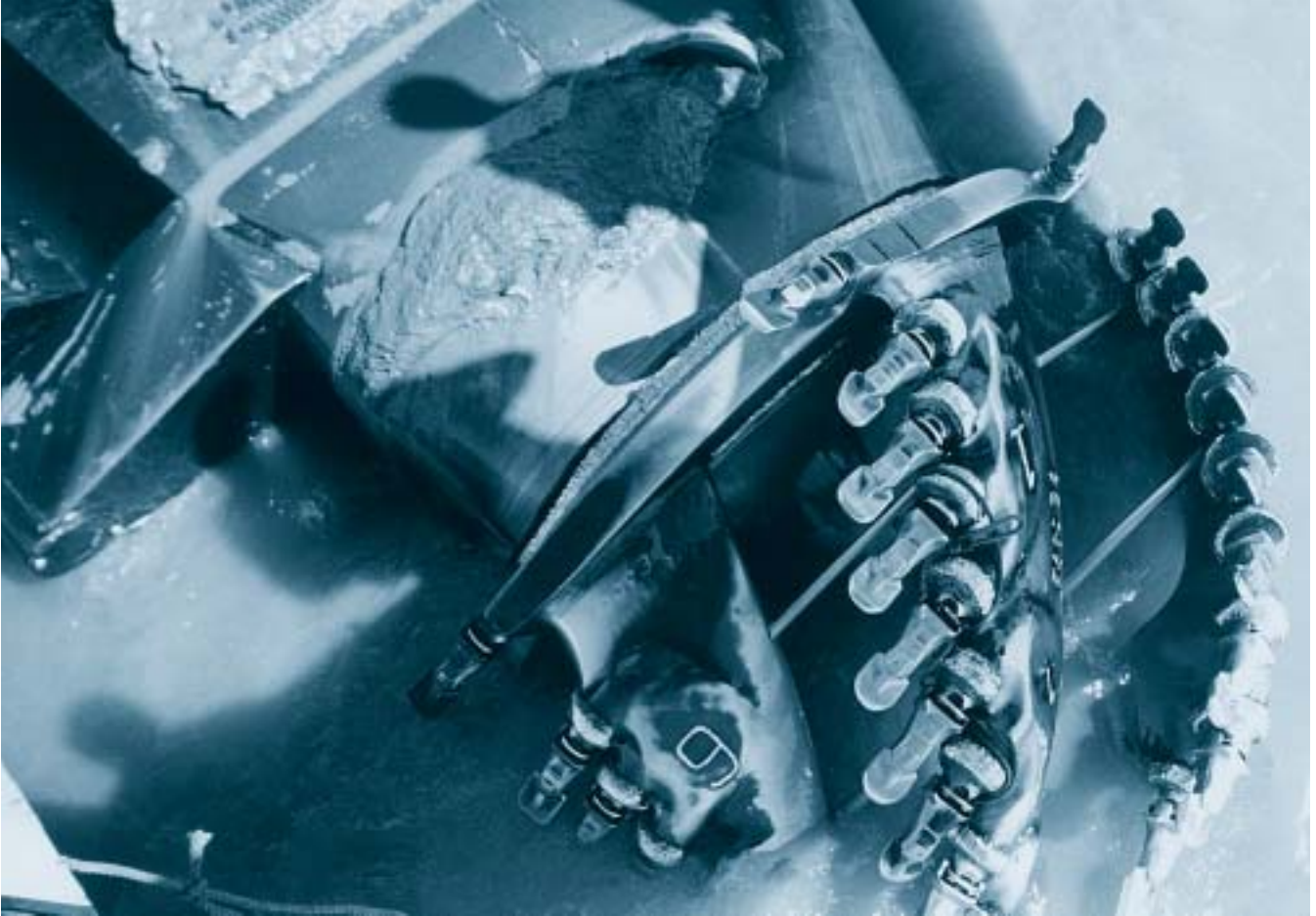
Figure 5. Cutting through hard rock demands specially developed cutter heads that can withstand incredible wear and tear.
