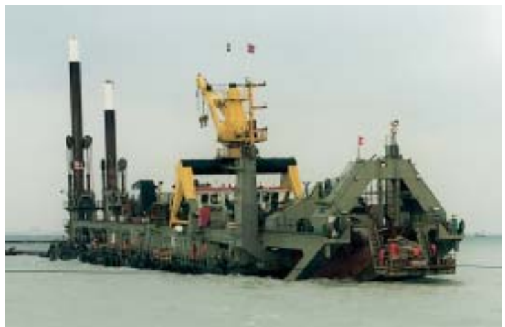
Figure 4. The cutter suction dredger Castor, at work in the Øresund, is equipped with innovative anchoring systems and precision excavation control.
