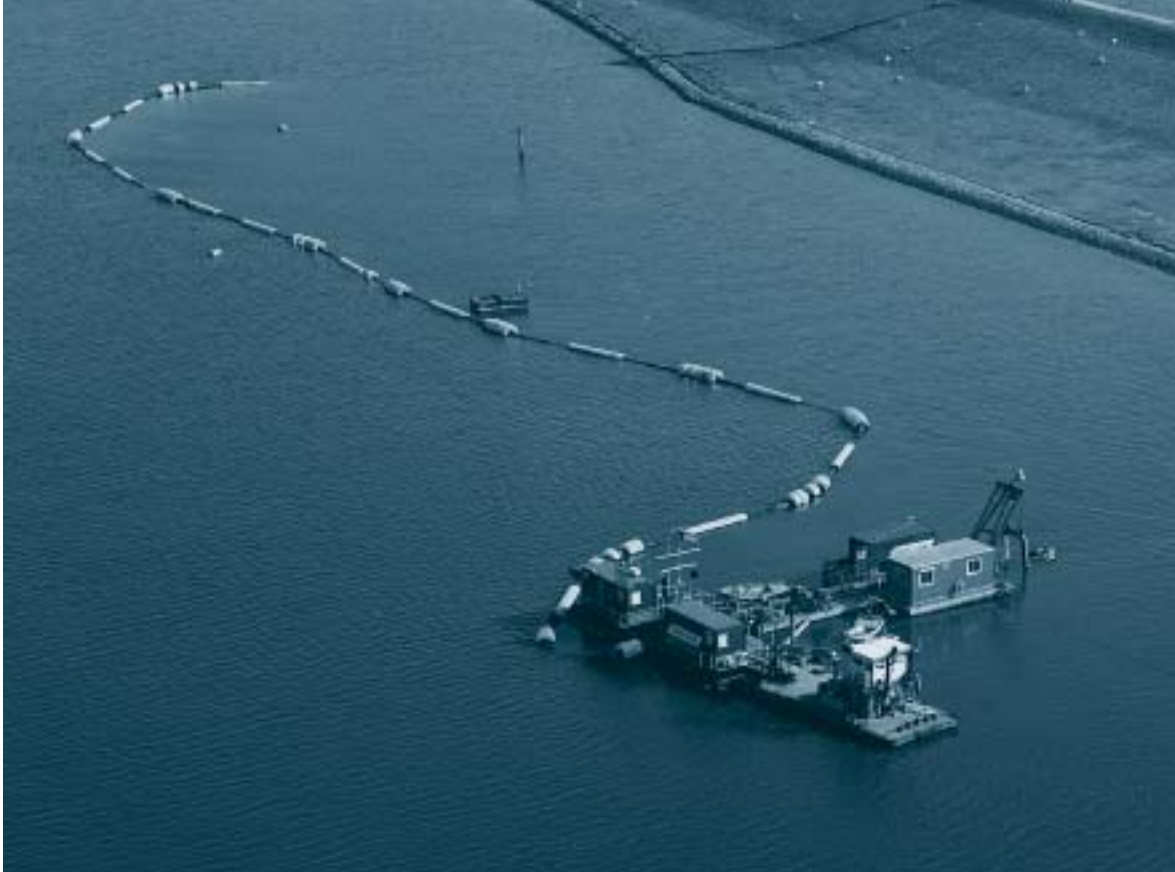
Figure 7. Specialist dredgers such as this auger dredger at work in the harbour of Delfzijl, The Netherlands handle smaller quantities of sediment but are equally important.
