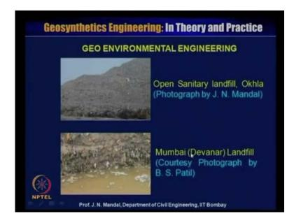
So, you require proper kind of the geosynthetic material to control the Tsunami disaster, the next I will just address some of geoenvironmental engineering. You can see that, a kind of the landfill, this is open sanitary landfill in Okhla, huge landfill, it is open, it contaminated the ground surface. So, you require proper kind of covering, proper kind of scientific landfill systems should be, otherwise you can see, what is the kind of the problem, it is absolutely open.
