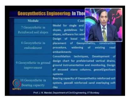
Module 7, geosynthetics in reinforced soil slope, it cover model for single and multi layer reinforced slope, guidelines for design of reinforced slope, software for reinforced soil slope. Module 8, geosynthetics in embankment, design of basal reinforced embankment, placement of geosynthetics, construction procedure, widening of existing road embankment.
