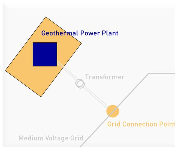
**Figure 20 Allocation of the grid connection point. Best-case-scenario: connection of the power plant to electricity grid by using the shortest distance (linear distance).**
