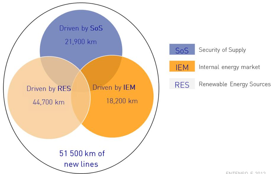
**Figure 10 Main drivers for investment in new or refurbished power lines (ENTSO-E, 2012)**
