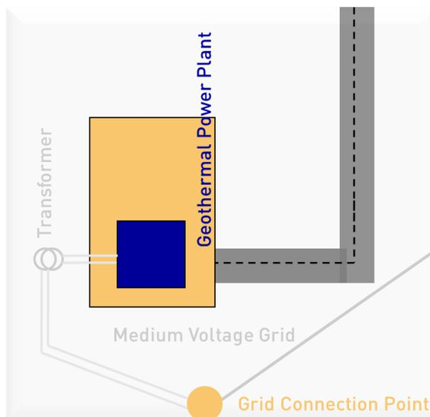
**Figure 22 Allocation of an alternative grid connection point. The nearest (linear distance) grid connection point is unsuitable due to economic issues.**
