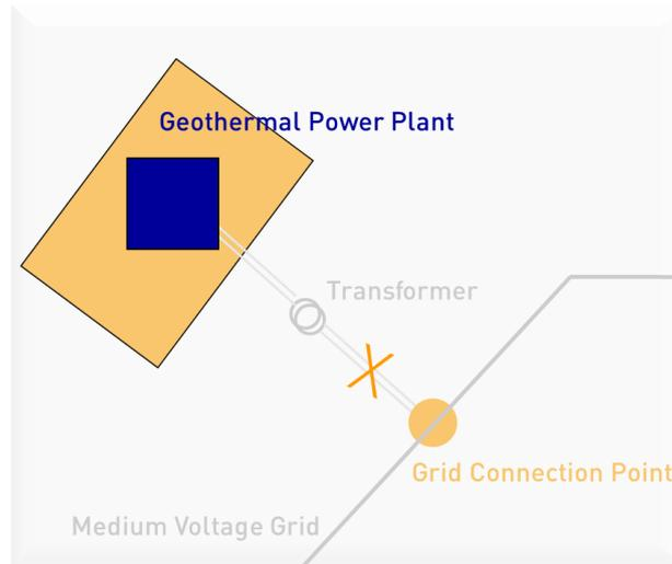
**Figure 21 Allocation of the grid connection point. The nearest (linear distance) grid connection point is unsuitable due to technical issues.**
