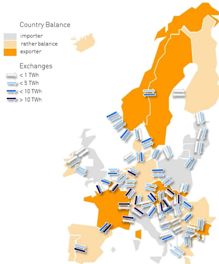
**Figure 11 Power exchange pattern in 2020 between the ENTSOE member states (ENTSO-E, 2012)**
