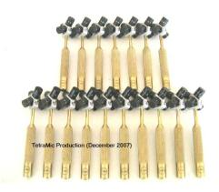
Figure 2.4: TetraMic from *Core Sound* [7], which delivers signals in A-format, and they have to be converted to B-format externally.
