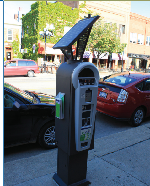
A solar-powered multispace parking meter in Ann Arbor, Michigan. (Credit: Dwight Burdette / Creative Commons 3.0)
