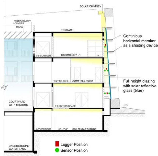
Figure 2 Solar chimneys on the façade and misters in the courtyard in building W2
