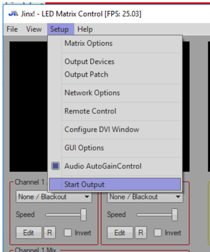
At this point the leds on Arduino Uno will start to flash and you led panel will get black.
