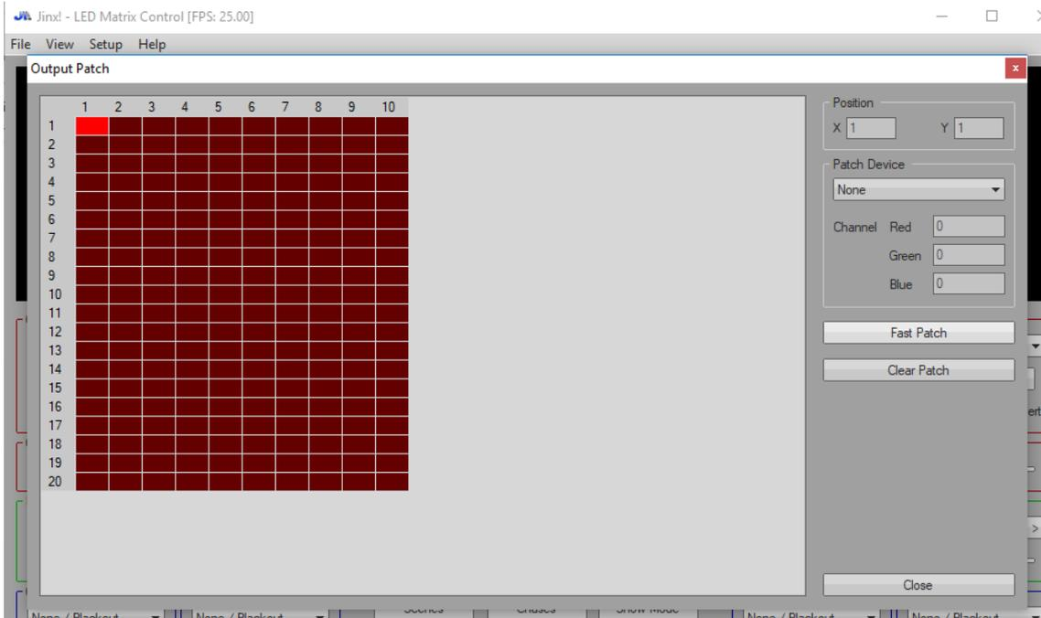
As you can see, I have a 10 x 20 panel as informed on Matix Options. If you have a bigger matrix and want to use more than one Arduino, you have to set up the parts of the whole panel for each Arduino. In my case it is only one Arduino, so click on Fast Patch.
