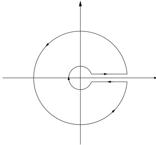
FIGURE 4. Contour for integrals involving branch cuts
