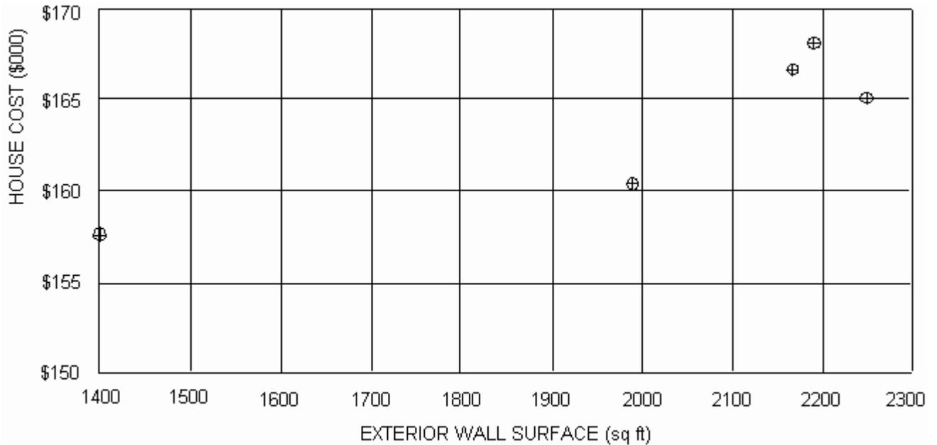
**Step 5. Select the relationship that best predicts the dependent variable.** Based on the initial analysis, it appears that square feet of living area and exterior wall surface have the most potential for development of a CER. The two graphs below depict efforts to fit a straight line through the observed values. Note that both graphs demonstrate efforts to fit a line with and without using the data from the Ambassador model.
