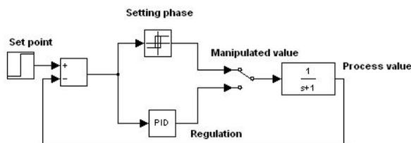
Fig. 2: The principle of the relay method.
