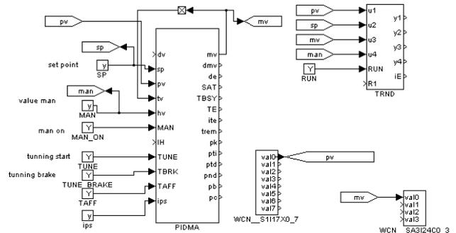
Fig. 7: Simulation scheme with PIDMA function block.
