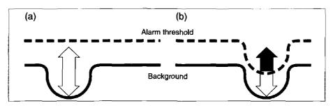
FIG. 1. Principle of background suppression. (a) Fixed threshold, signal ignored; (b) adaptive threshold, signal recognized.
