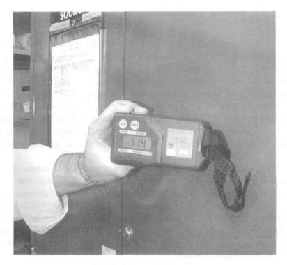
FIG. 2. Gamma densitometer.
