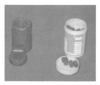
FIG. 1. Illicit uranium cylinder (with lead pig) (left) and reactor fuel pellets (right)
