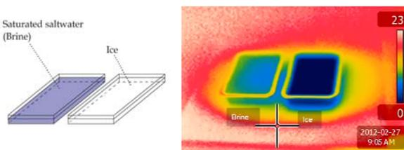
*Figure 9: This thermogram shows (unfrozen) saltwater warmed up more quickly than ice. Their initial temperatures were the same.*
