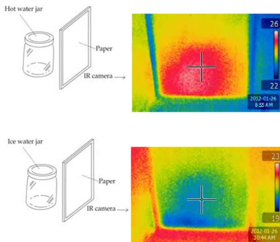
Figure 5: Radiation heat transfer between a hot water jar (~70°C) and a paper screen (upper images) and between an ice water jar (~5°C) and a paper screen (lower images).
