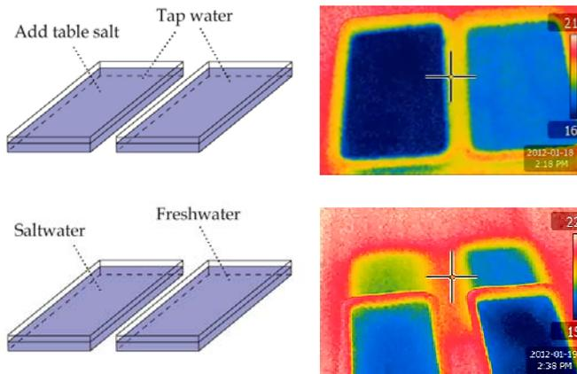
Figure 7: The upper images show water cooled down when salt was added. The lower images show, after the salt was completely dissolved, that the saltwater became warmer. (The lower thermogram shows that the foam board surface below the freshwater container was also cooler, suggesting that this effect was not due to a possible difference in emissivity, if any, caused by the added salt ions.)
