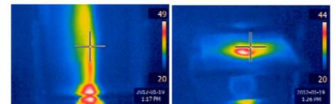
*Figure 4: A screen to capture the three-dimensional heat flow through natural convection from a heater.*
