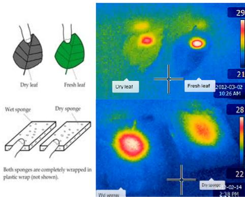
*Figure 3: These two experiments compared the heat transfer from fingers to a dry leaf and a fresh leaf (upper) and to a wet sponge and a dry sponge (lower). It was shown that more heat transferred to a fresh leaf than to a dry one, and to a wet sponge than to a dry one, suggesting the role of water content on storing thermal energy.*
