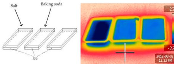
*Figure 8: This thermogram shows that adding salt to ice resulted in cooling that was much more significant than adding baking soda to ice.*
