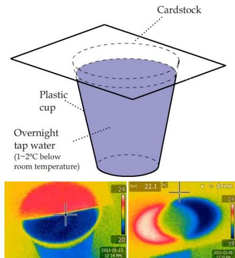
*Figure 11: A piece of paper or cardstock warmed up when it was put above a cup of water. Shifting it resulted in a thermogram that simultaneously showed heating and cooling related to latent heat.*
