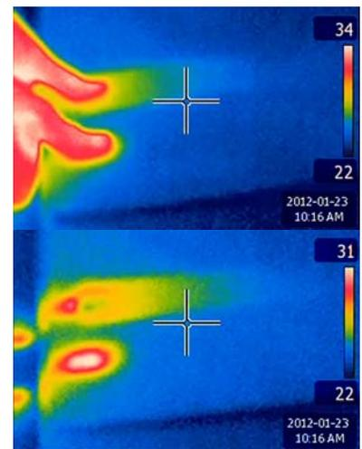
*Figure 1: This experiment shows a comparison of thermal conductivities of metals and foams. A thin aluminum strip was placed on top of a foamcore board. They were covered up by a piece of paper to eliminate the effect of different emissivities of the metal and the foam. The two fingers were used as identical heaters.*
