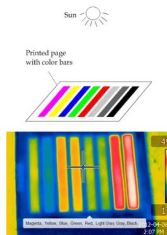
Figure 6: Comparing light absorption of different colors.
