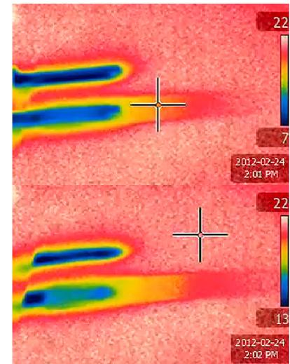
*Figure 2: This experiment is approximately opposite to the one described in Figure 1. Thermography creates an illusion as if cold could also flow just like heat. In the upper thermogram, the two cold pieces were laid on the setup. In the lower one, they had been removed.*
