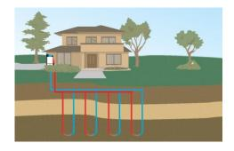
Figure 12: Geothermal Vertical Loop (GeoComfort, 2008)
