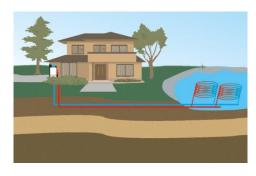
Figure 14: Geothermal Pond Loop (GeoComfort, 2008)
