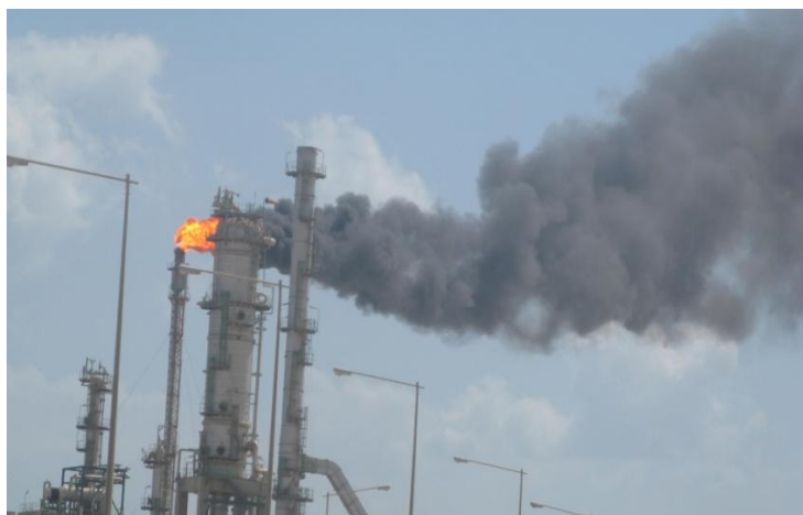
Figure 2: Uncontrolled flaring without steam
