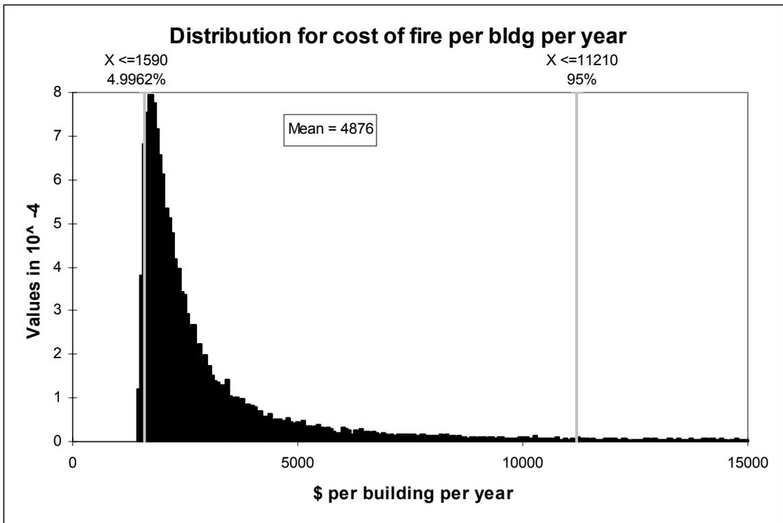
Figure 39. Model output distribution for cost of fire per building per year – with detection
