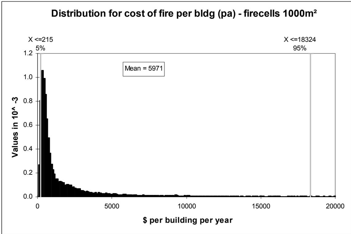
Figure 40. Model output distribution for cost of fire per building per year – with fire cells max 1000 m<sup>2</sup>
