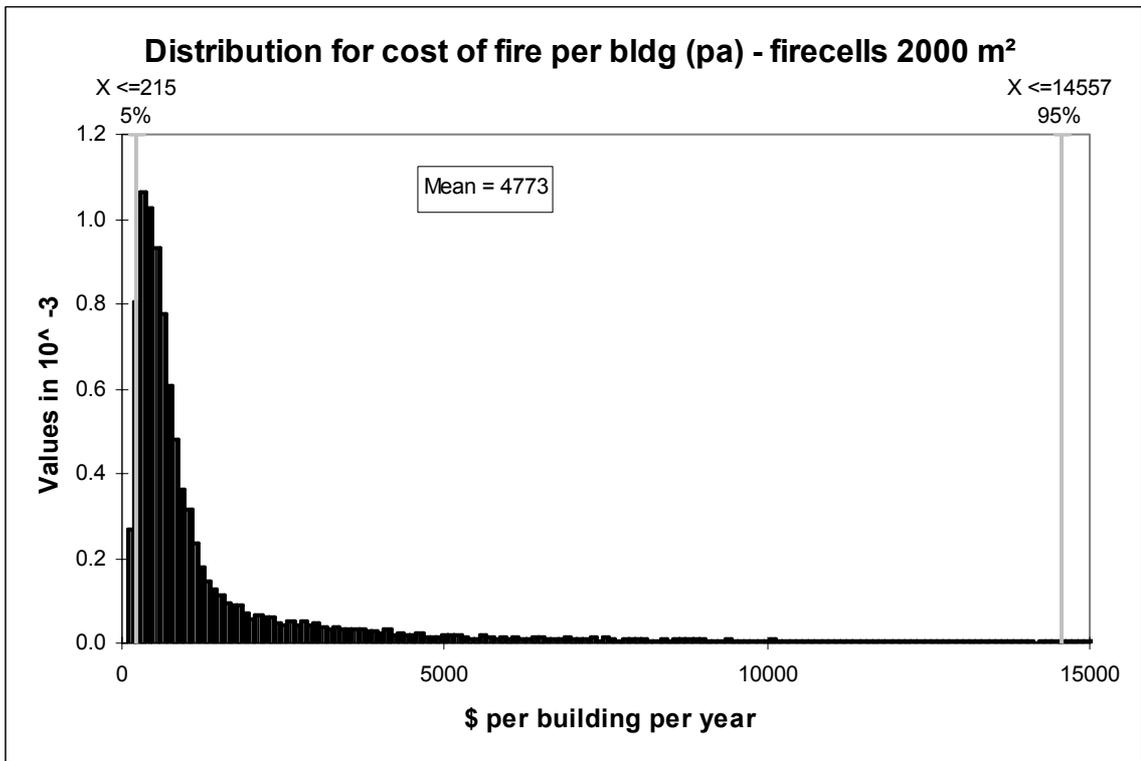
Figure 41. Model output distribution for cost of fire per building per year – with fire cells max 2000 m<sup>2</sup>
