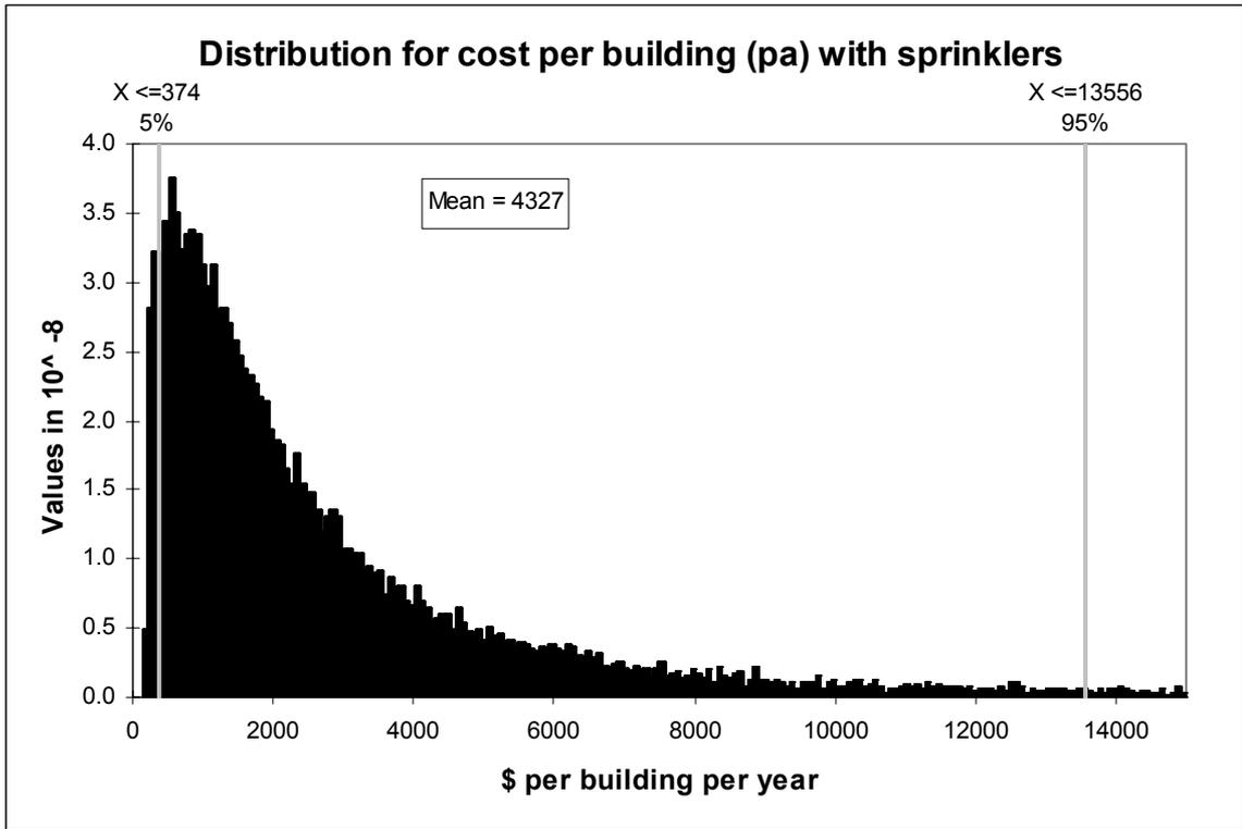
Figure 38. Model output distribution for cost of fire per building per year – sprinklered building
