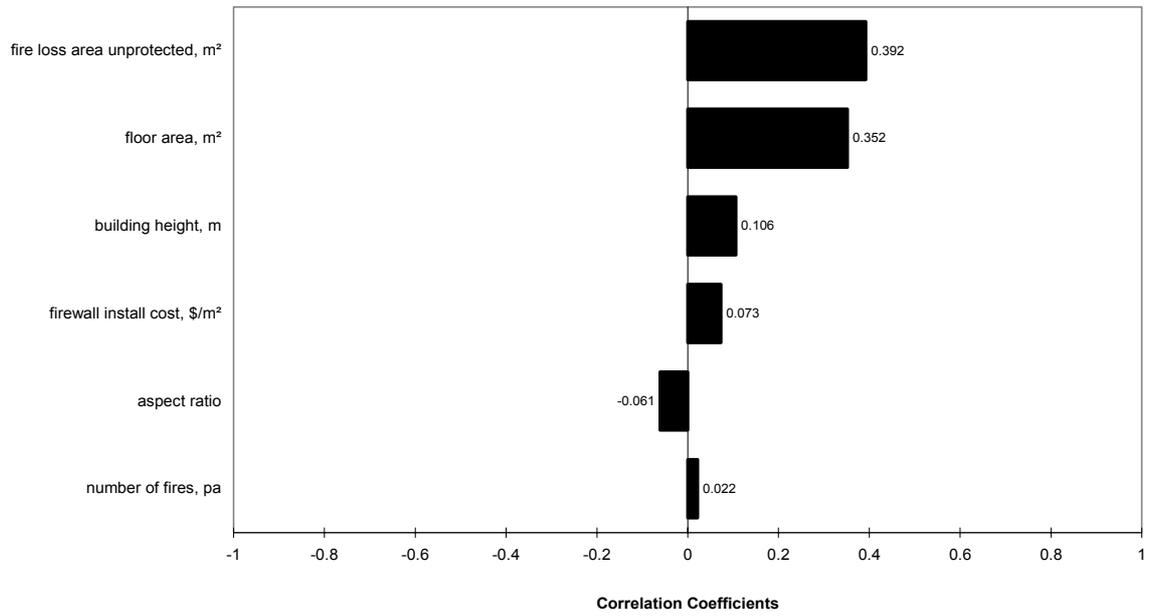
Figure 47. Tornado chart for compartmented buildings (1000 m<sup>2</sup> fire cells)
