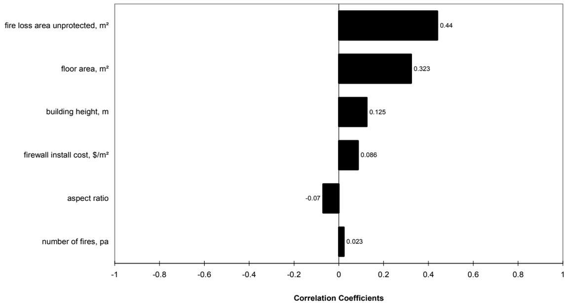
Figure 48. Tornado chart for compartmented buildings (2000 m<sup>2</sup> fire cells)
