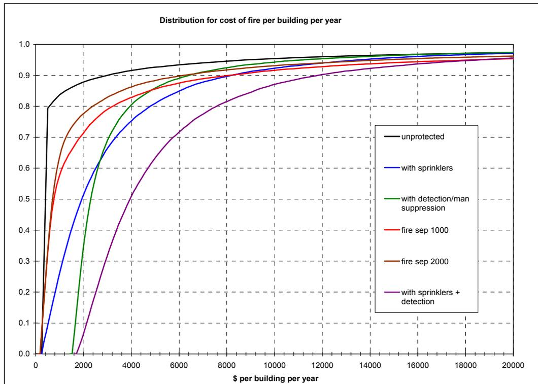
Figure 43. Comparison of ascending cumulative frequency for the cost of fire per building (pa) of different fire protection options
