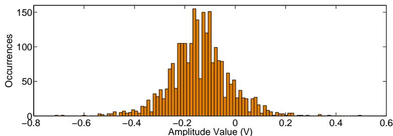
Figure 3: Histogram of Chaotic Photovoltaic Output
