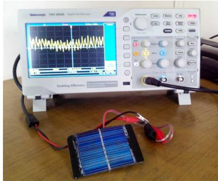
Figure 1: Experimental setup to characterize photovoltaic voltage
