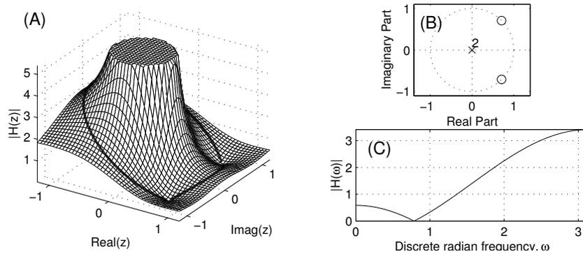
Figure 9.2: (A) The  $z$ -plane surface defined by the system function  $H(z) = (1 - e^{j\pi/4}z^{-1})(1 - e^{-j\pi/4}z^{-1})$ . (B) The corresponding pole-zero plot. (C) The corresponding magnitude frequency response.
