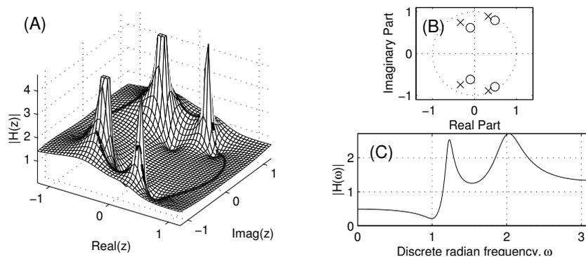
Figure 9.4: (A) The  $z$ -plane surface for a complicated system function with four poles and four zeros. (B) The corresponding pole-zero plot. (C) The corresponding magnitude frequency response.
