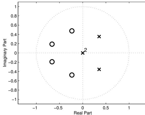
Figure 9.1: A pole-zero plot of an IIR filter.
