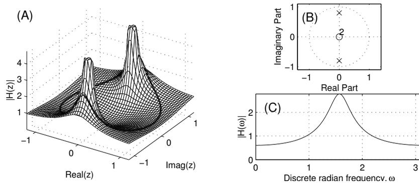
Figure 9.3: (A) The  $z$ -plane surface defined by the system function  $H(z) = \frac{1}{(1-0.8e^{j\pi/2}z^{-1})(1-0.8e^{-j\pi/2}z^{-1})}$ . (B) The corresponding pole-zero plot. (C) The corresponding magnitude frequency response.
