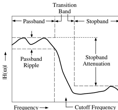
Figure 9.5: An illustration of the various bands of a lowpass filter.
