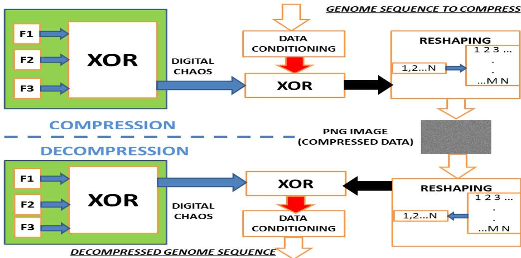
Figure 1 Block Diagram illustrating the proposed Genome Data Compression Technique
