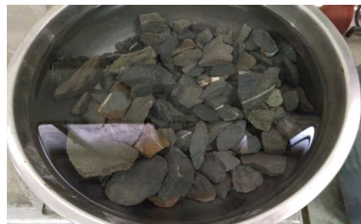
Figure 7 Coarse aggregates submerged in water
