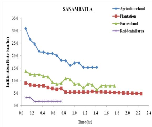
Figure.3 Infiltration capacity curve for sanambatla village
