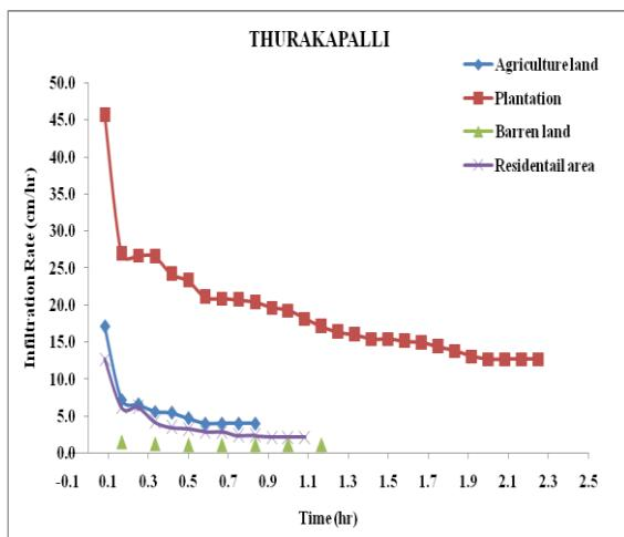
Figure.4 Infiltration capacity curve for Thurakapalli village
