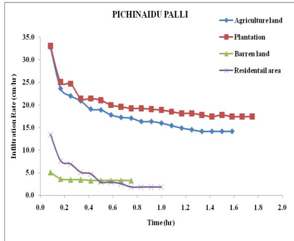
Figure.5 Infiltration capacity curve for Pichinaidupalli village
