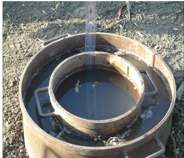
**Figure.2. Simple Double Ring Infiltrometer**
