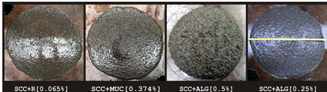
Fig.2.2 Visual appearance of SCC mixtures containing nopal mucilage and marine brown algae extract and a commercial viscosity modifying admixtures during the flow spread test at room temperature [Martinez et.al – 2014].
