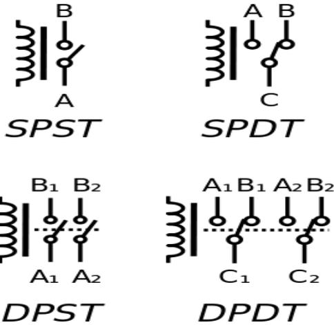
Fig.1 Types of switches
