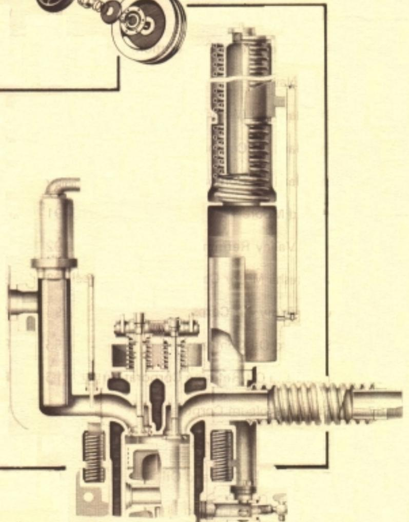
This cross section of the combustion chamber area of a motor method CFR engine shows a segment of the engine which has remained unchanged since development of the first model.
