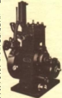
Figure 3—Fixed Compression Engine showing Battery Ignition System, Steam Cooling Condenser, and Water Pump.
