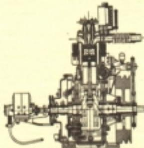
Figure 6 — Side Section of Variable Compression Engine
