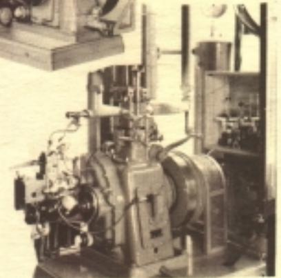
The supercharged version of the CFR engine shown above was used for rating aviation gasoline. Developed during World War II, this engine helped in the production of the Allies' superior aviation fuel, which was a decisive factor in winning the war.
