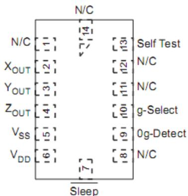
Figure.3.3 pin diagram of accelerometer
