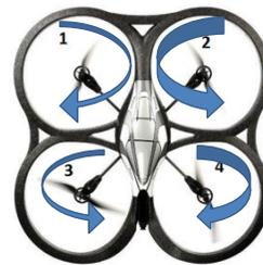
**Fig5. Move towards low speed motors**
