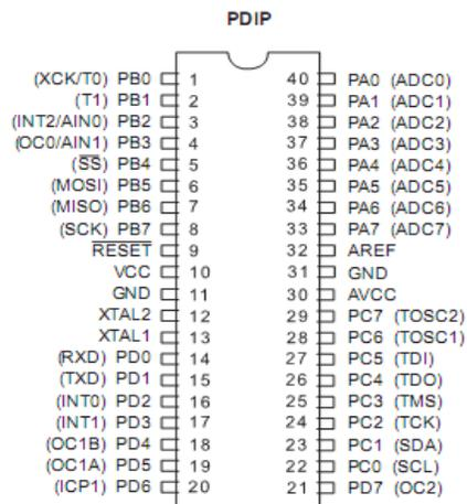
Figure.3.7 pin diagram of ATmega16
