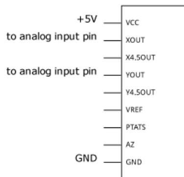
Figure.3.5 pin diagram of gyro
