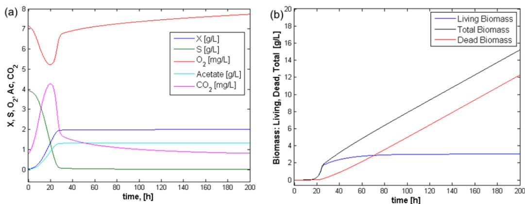
Figure 2: Time profile of live biomass, substrate, dissolved oxygen, dissolved CO<sub>2</sub>, acetate (a) and biomass growth, biomass death and overall development of a biofouling layer (b).
