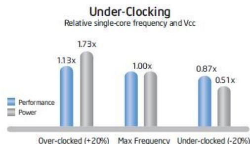
**Figure.1 Performance relative to power consumption in single core**
