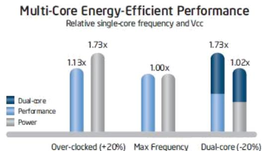
**Figure.2 Performance relative to power consumption in multi-core**
