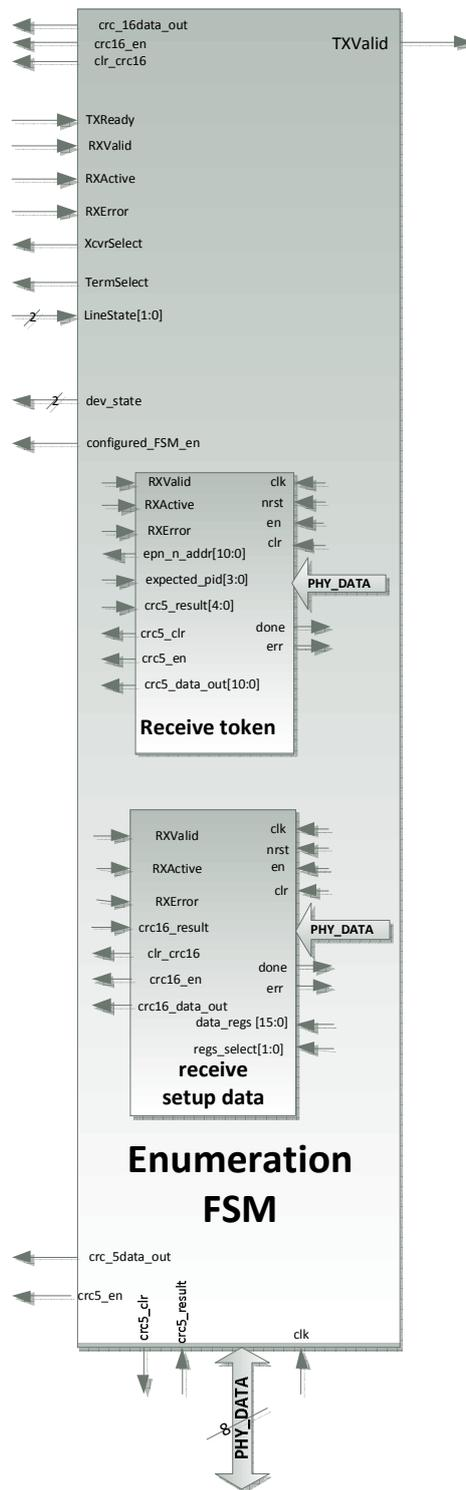
Figure 12 -Enumeration FSM block diagram.
