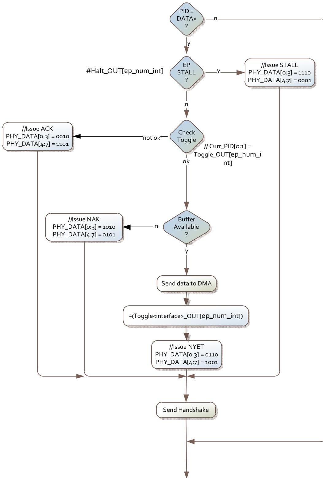
**Figure 40 - Bulk OUT Transfer state machine**
