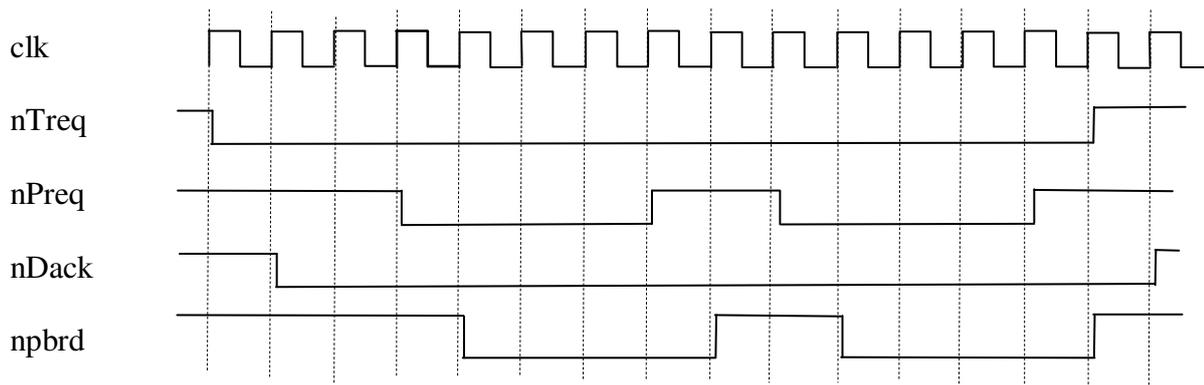
Figure 29- DMAC handshake signaling during an OUT transaction. Two packet transfers in one transaction.
