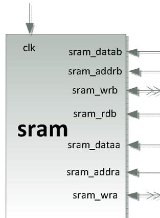
Figure 20 – SRAM block diagram.
