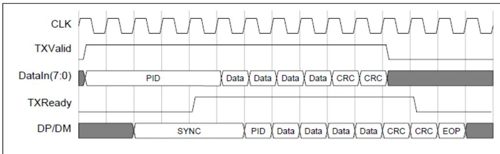
**Figure 32 - UTMI transmit signals timing**
