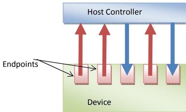
**Figure 1- Each endpoint supports data flow in one direction: either input (from device to host) or output (from host to device).**
