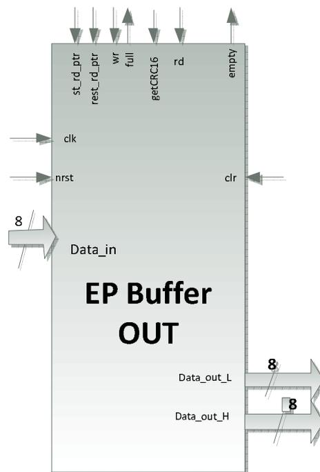
Figure 21 - EP Buffer OUT module block diagram
