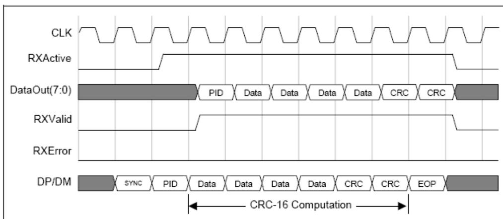
Figure 27- UTMI receive signals timing
