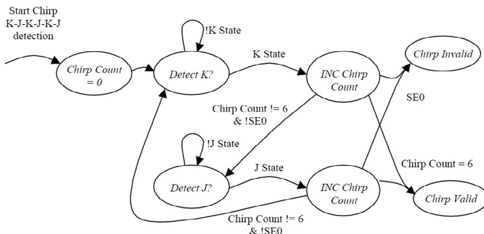
Figure 13 - High speed detection state machine
