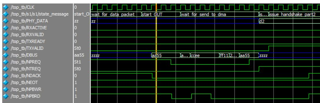
Figure 34 – Packet is sent to the DMA in an OUT transaction.
