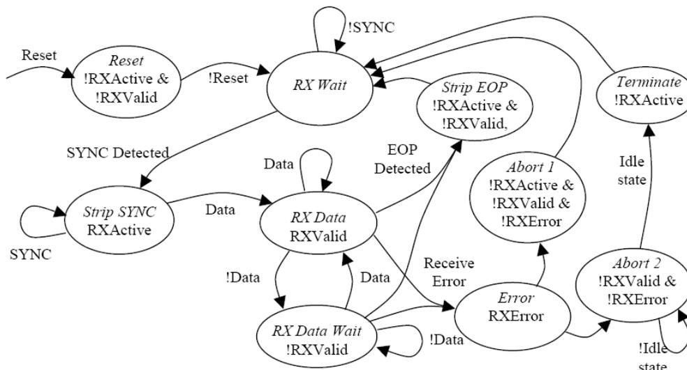
Figure 26- UTMI Receive State Diagram
