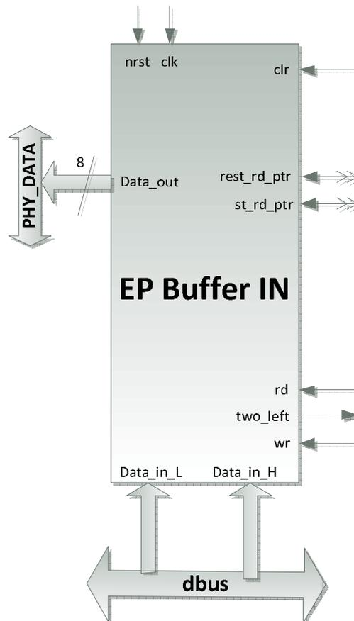
Figure 22 - EP Buffer IN module block diagram
