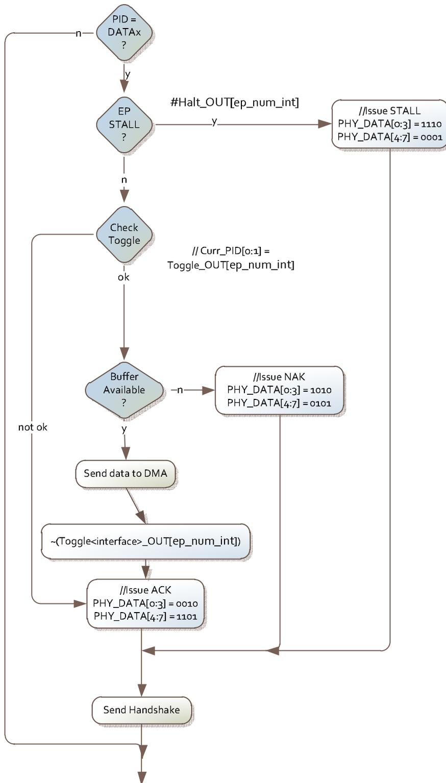
**Figure 41 - Interrupt OUT Transfer state machine**
