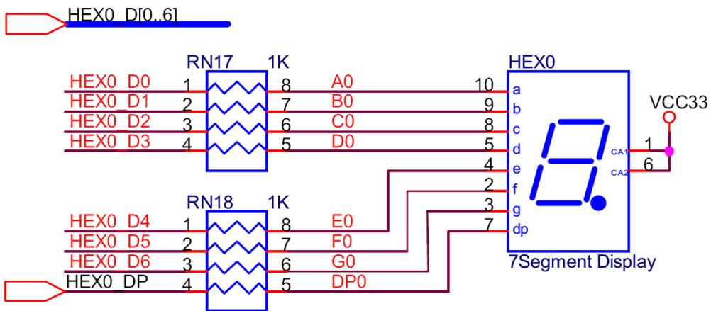
**Figure 37 - Schematic diagram of the 7-segment displays**
