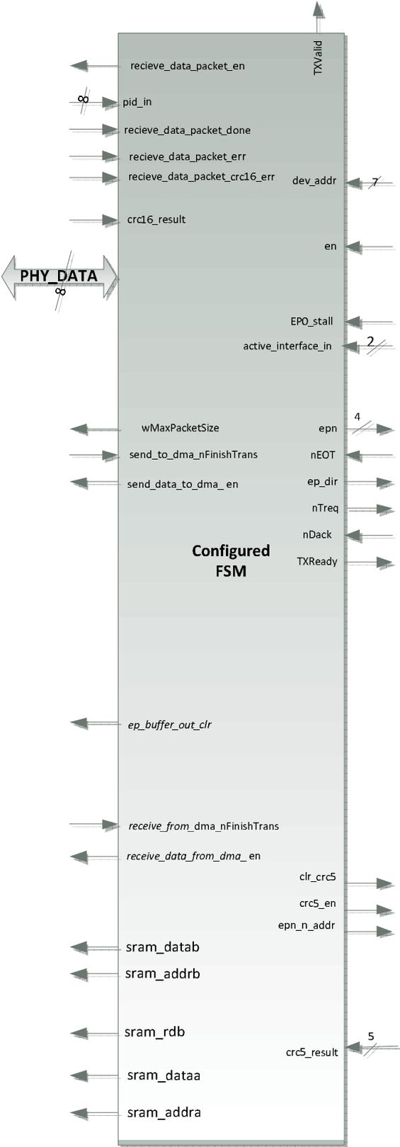
Figure 16 –Configured FSM block diagram.
