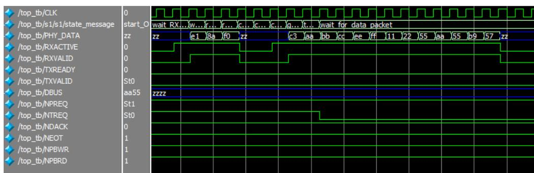
Figure 33 - Packet received from the UTMI in an OUT transaction.
