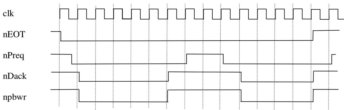
**Figure 31– DMAC handshake signaling during an IN transaction. Two packet transfers in one transaction.**
