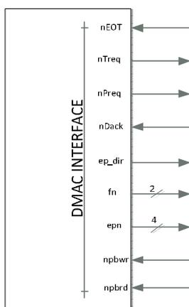
Figure 10 – DMA Interface Block diagram.
