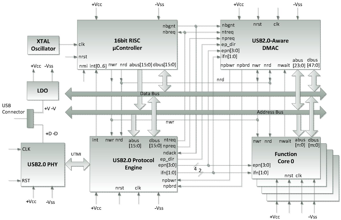
Figure 8 - μController-based Device Controller Block Diagram
