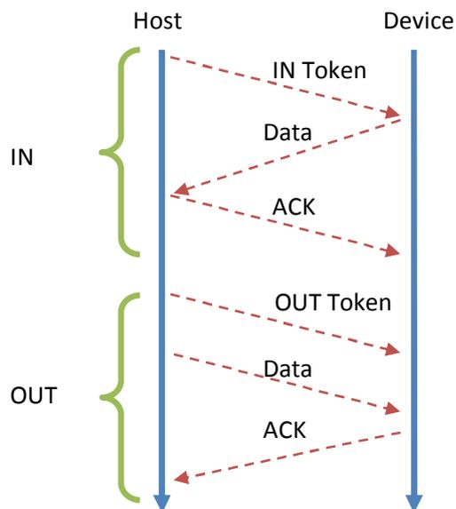
**Figure 4 - A typical USB transaction involves a token packet followed by a data packet and ends with a handshake packet**
