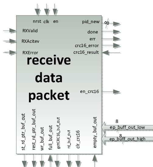
Figure 17 – Receive Data Packet block diagram.
