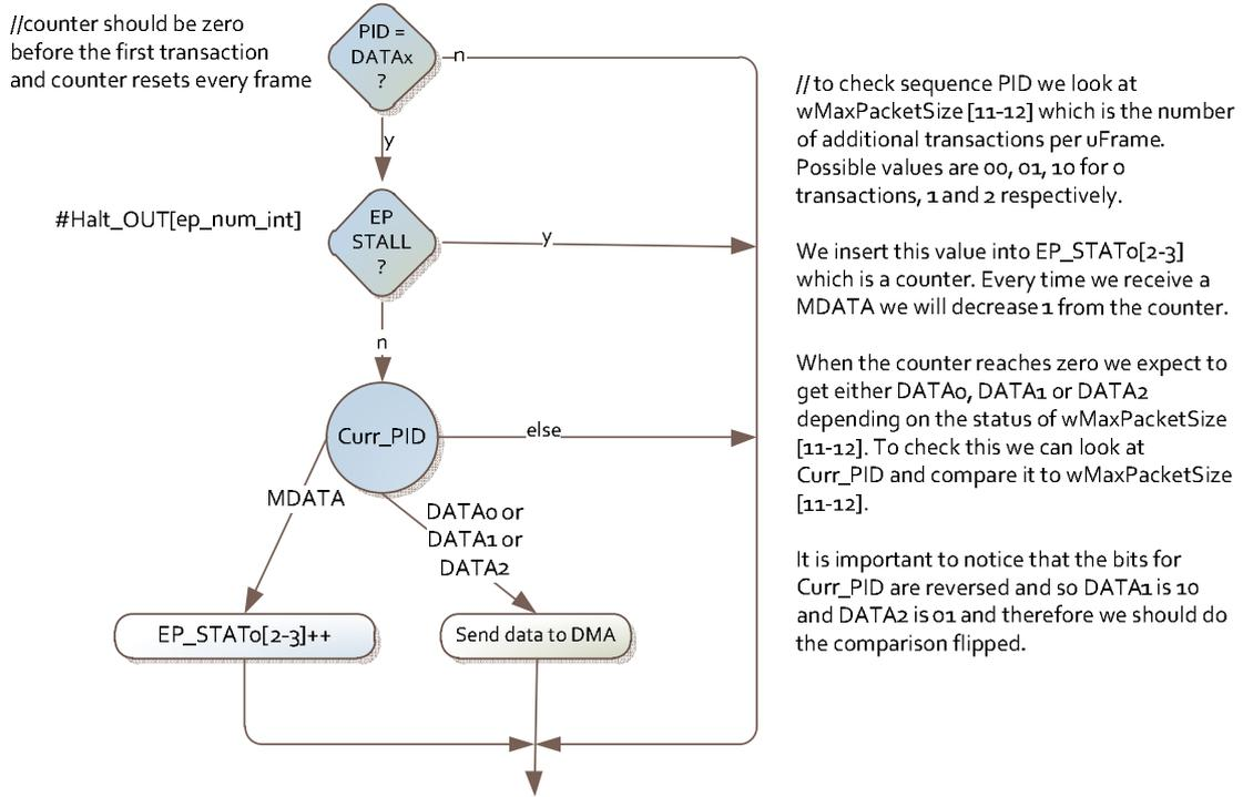
Figure 42 – Isochronous OUT Transfer state machine
