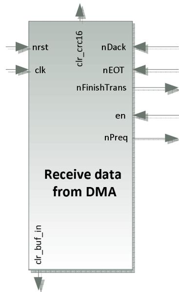
Figure 19 - Receive Data from DMA block diagram.
