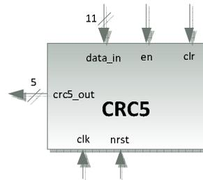
Figure 23 – CRC5 module block diagram
