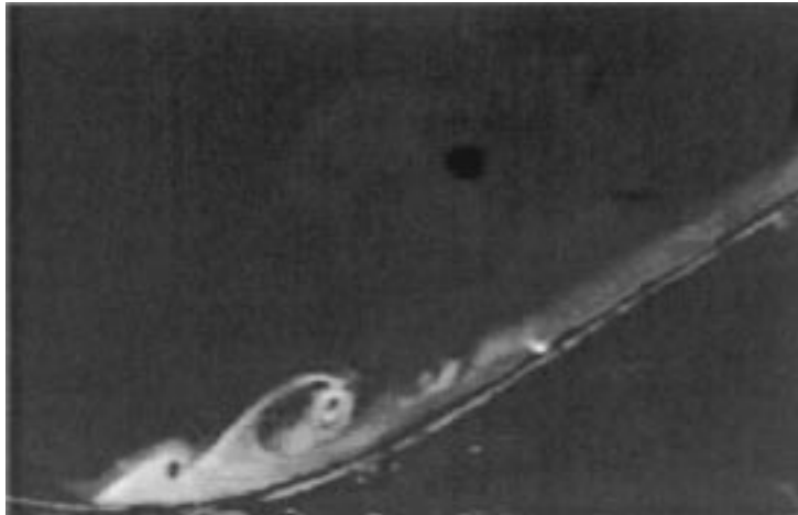
Figure 12. Laboratory experiment designed to simulate katabatic flow in a basin. Note the down-slope flow into the basin. The shear between the katabatic flow and the turbulent fluid generates overturning instabilities. The laboratory experiments shown in Figures 12 and 13 were carried out at Arizona Sate University.
