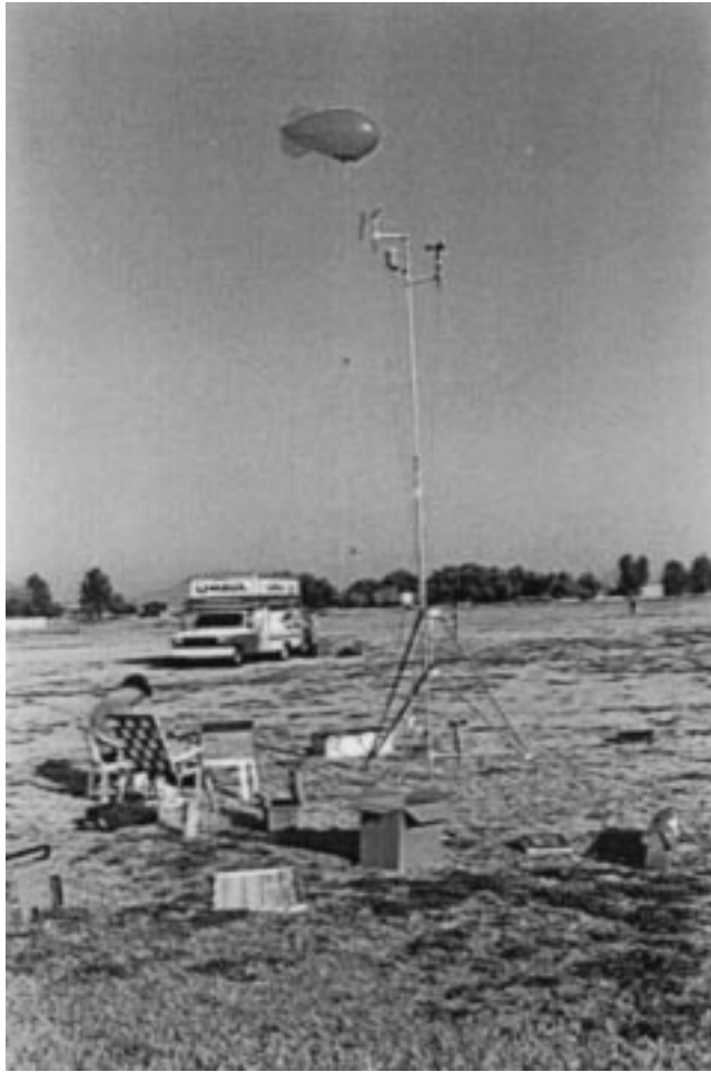
Figure 15a. A photograph showing the PAFEX-I instrumentation. It consists of a tethered meteorological tower carrying the sondes and a ground meteorological station. (b) A ‘streaker’ suspended from the meteorological tower.
