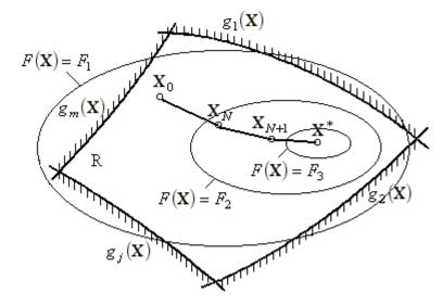
Fig. 1. The two-dimensional space of control variables of system, that is subjected to optimization
