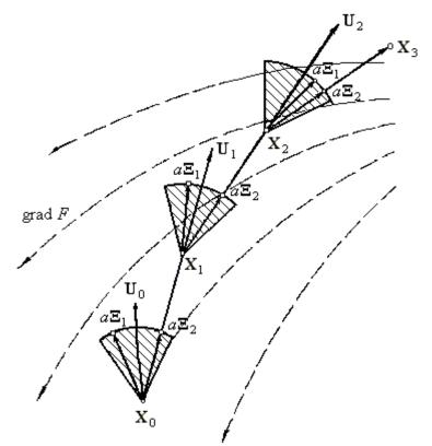
Fig.3. The algorithm with the guide cone. The motion of system in the space parameters of optimization
