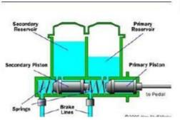
The diagram of master cylinder is shown in figure.
