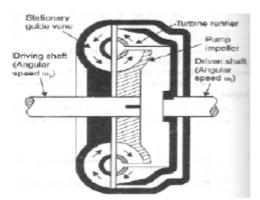
Hydraulic torque converter
