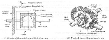
Whenever the car goes round a turn, the outer drive wheel travels a greater distance than the inner drive wheel. The two pinion gears rotate on their shaft and send more rotary motion to the Outer wheel. The gear ratio in the differential is usually referred to as the axle ratio. However it Would be more accurate to call it the differential ratio.
