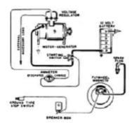
In magneto ignition system a magneto is used to generate electric current for producing spark. A high tension magneto generates a very high voltage needed for spark plug
