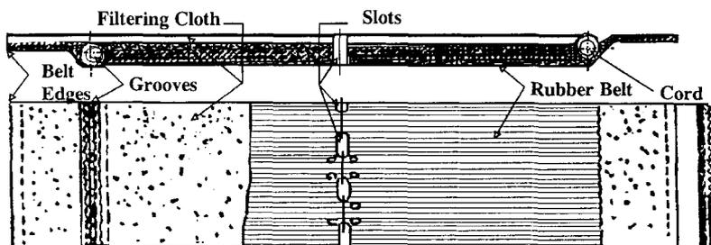
Figure 17. Filtering partition for a belt filter.
