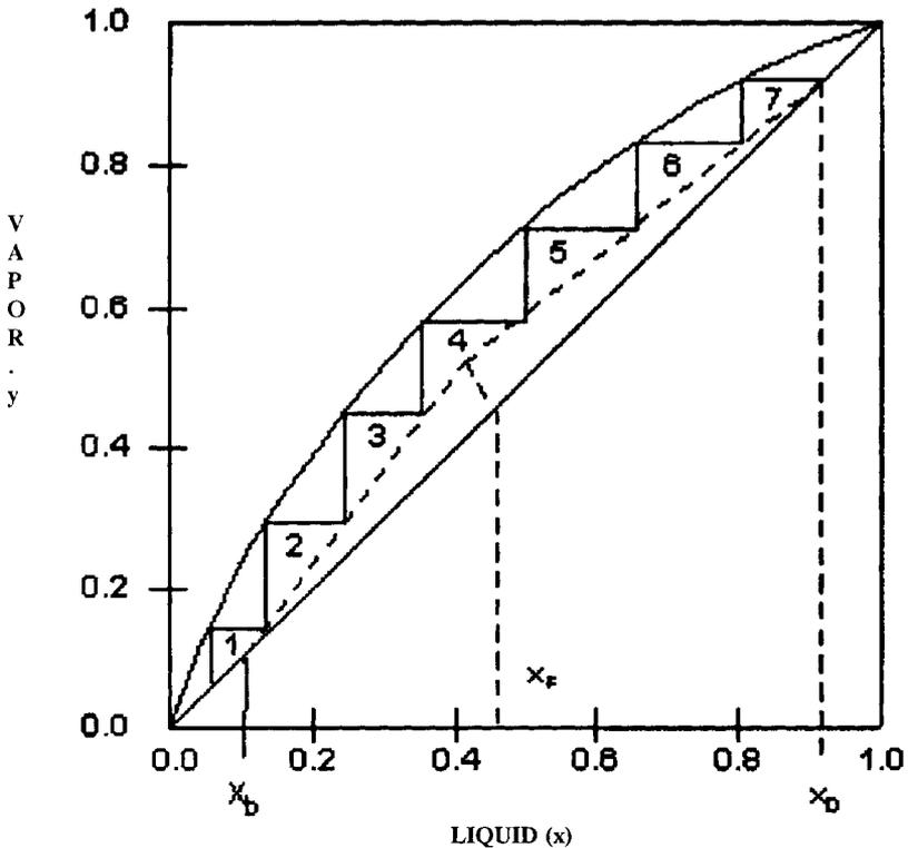
Figure 16. Example of a seven stage distillation.
