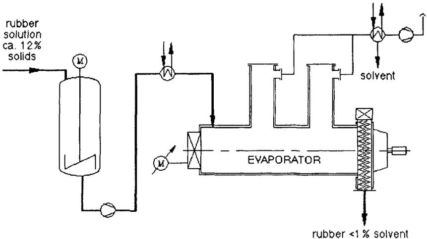
**Figure 17.** Process flow scheme for continuous evaporation in a rubber desolventizing process.
