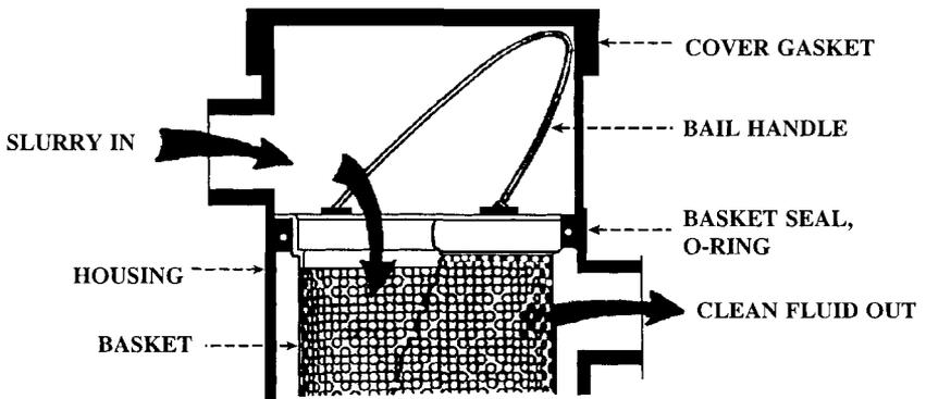
Figure 23. Upper portion of basket with seal.
