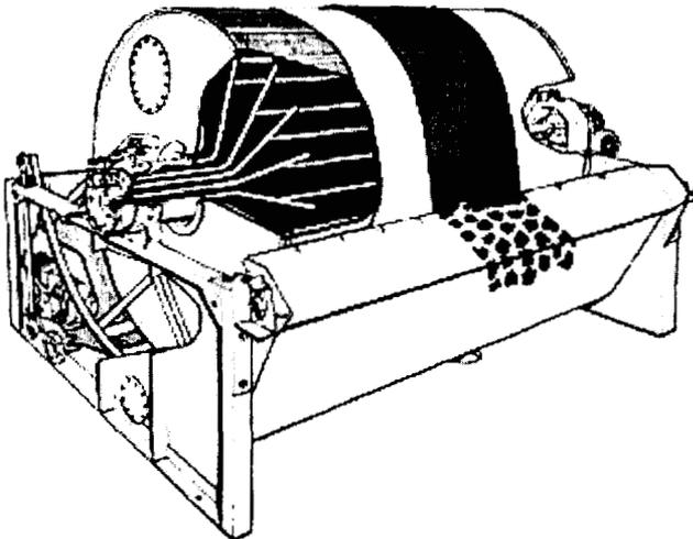
Figure 8. Rotary drum filter.
