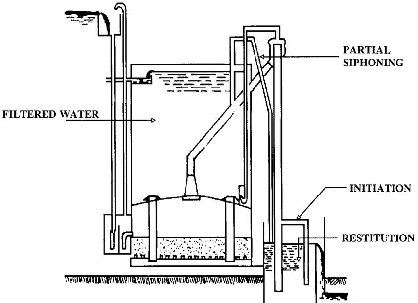
Figure 29. Automatic backwashing filter with a partial siphon.
