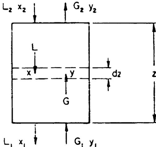
Figure 13. Differential mass balance definition.
