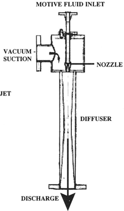
Figure 17. Jet vacuum pump.
