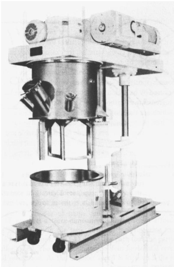
**Figure 5.** Planetary mixer with a vacuum hood.
