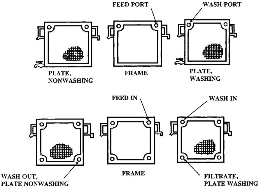
Figure 19. Plate and frames for open and closed delivery systems.
