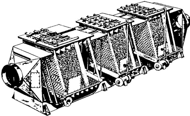
Figure 5. Example of multiple bed cross-flow scrubber.
