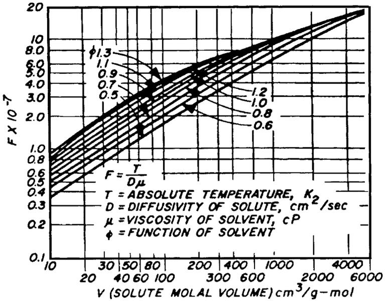
Figure 7. Solvent characteristic,  $F$ , versus solute molal concentration.
