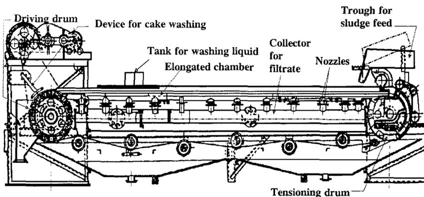
Figure 16. Basic design features of a belt filter.
