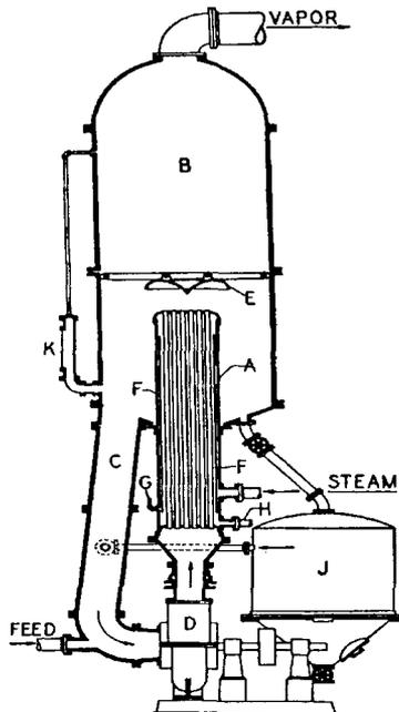
Figure 9. Forced circulation evaporator.
