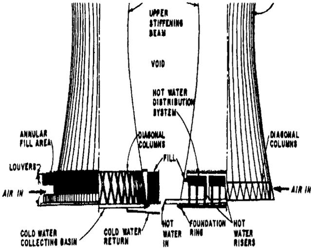
Figure 9. Compares cross flow and counterflow towers.
