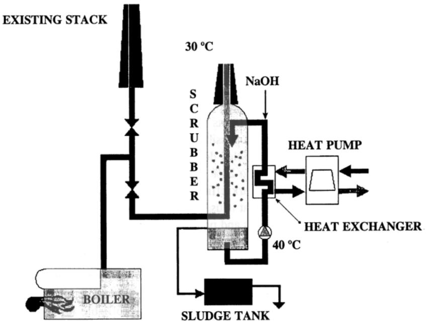
Figure 15. Example of a packaged flue gas scrubber system.
