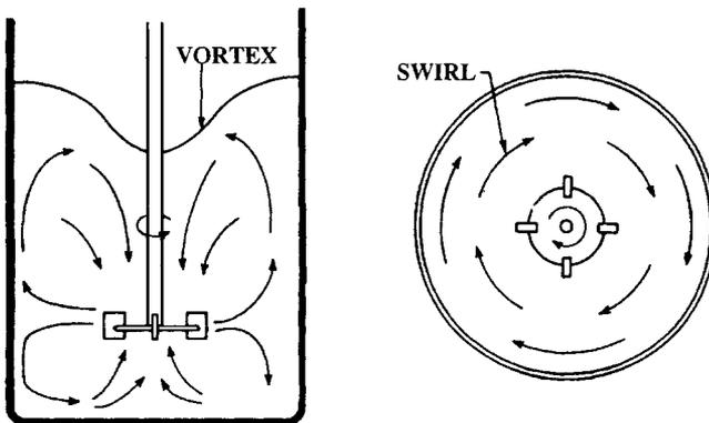
Figure 14. Circulation patterns in an agitated tank.
