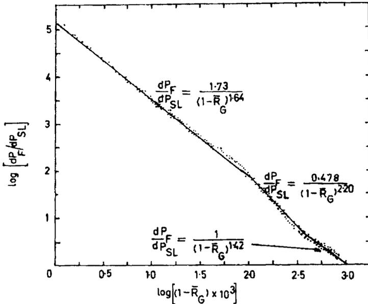
Figure 27. Empirical correlation between pressure drop and hold-up.
