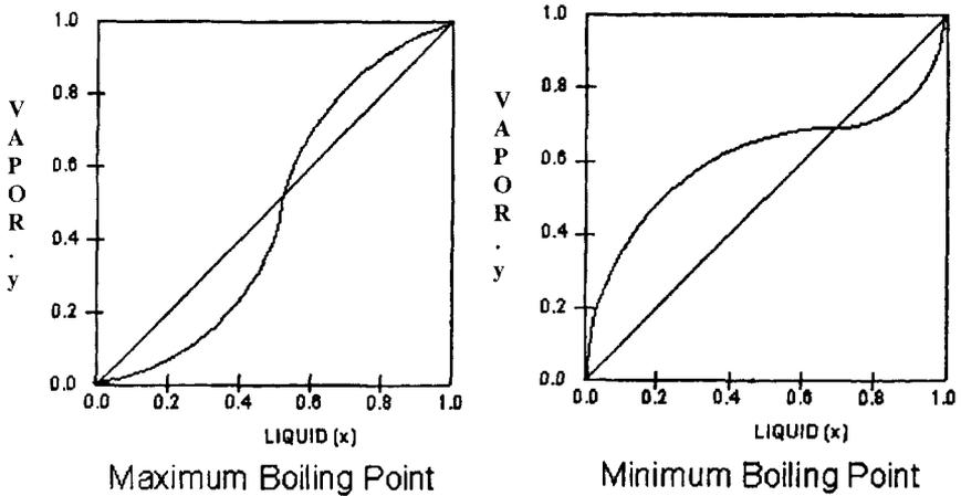
Figure 11. VLE curves for azeotropic systems.
