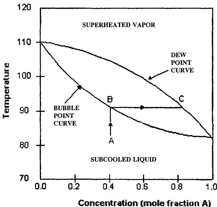
Figure 8. Boiling point diagram for binary mixture.
