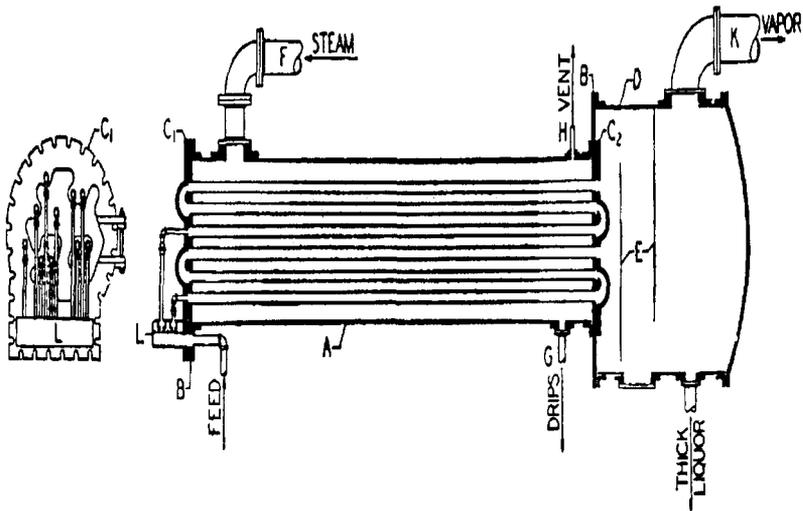
**Figure 13.** Steam outside tube evaporator: (A) Shell; (B) Tube sheets; (C<sub>1</sub>, C<sub>2</sub>) Distributing plates; (D) Vapor head; (E) Baffles; (F) Steam inlet; (G) Condensate outlet; (H) Non-condensed gas vent; (J) Thick liquor outlet; (K) Vapor outlet; (L) Liquor feed box.
