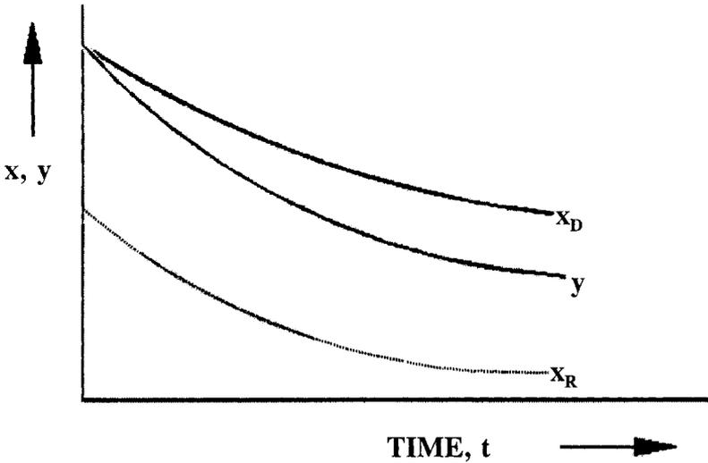
Figure 9. Dynamic equilibrium curve for batch distillation.
