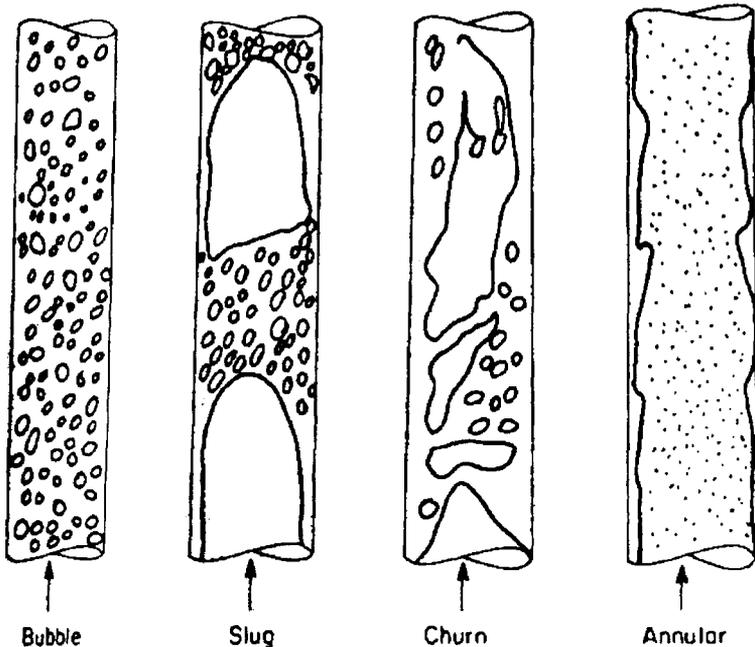
Figure 23. Flow patterns in vertical pipe flow.
