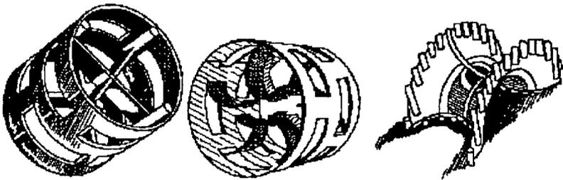
Figure 6. Sketch of common packing configurations.
