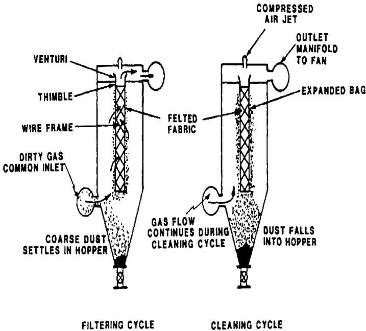
Figure 5. Automatic baghouse with pulse jet cleaning.
