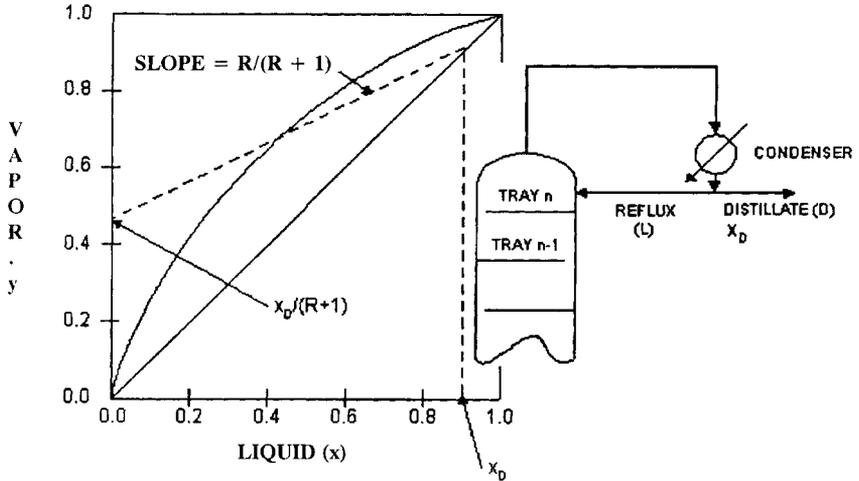
Figure 13. Application of McCabe-Thiele to VLE diagram.
