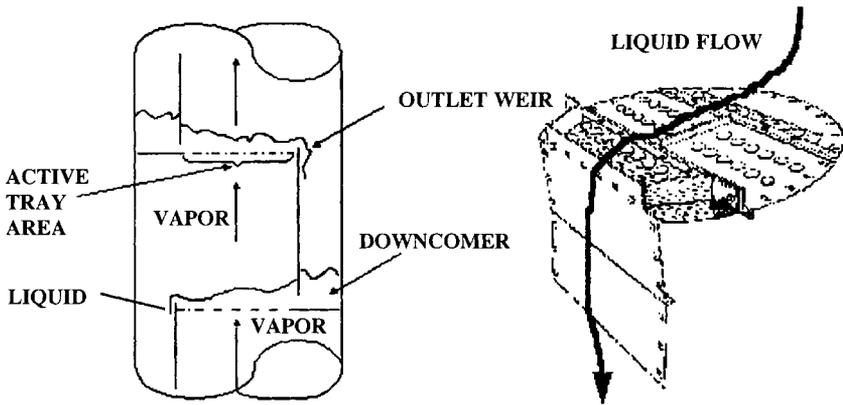
Figure 5. Downcomer operation and flow over a tray.
