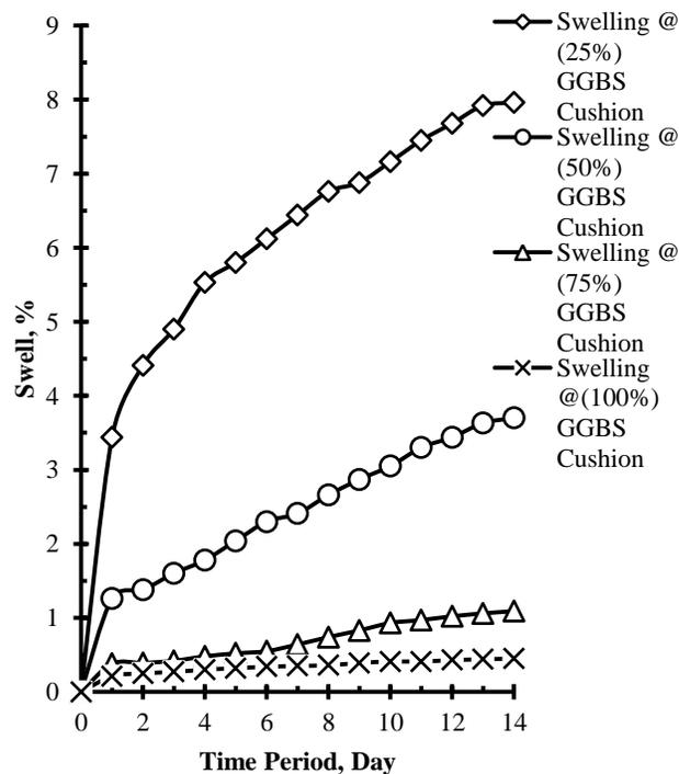
**Figure 2.** Swell behaviour of expansive soil with different thickness of lime treated GGBS cushion
