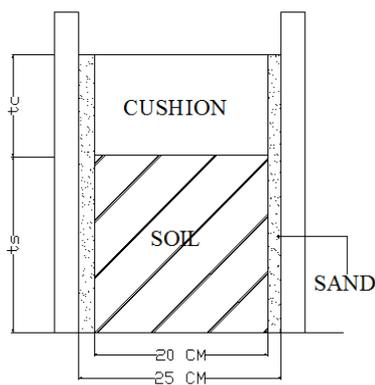
**Figure 1.** Schematic representation of sample preparation of soil-cushion layers for test
