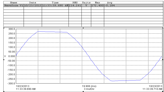
Fig. 19: Inverter system output voltage waveform with R.M.S value of 214V
