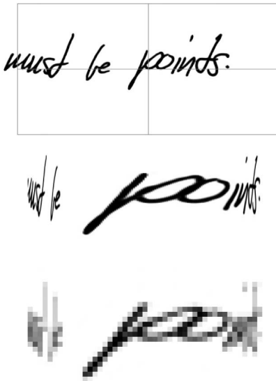
Fig. 6. Fisheye lens example (from up-to-down): original image of 500 \times 250 pixels centered at the pixel to be classified; the same image with a fisheye lens distortion; the image downsampled to 50 \times 30 values used by the neural network classifier.
