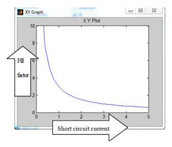
Figure 1. Fill factor effect on various levels of short circuit current
