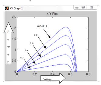
Figure 4. P-V characteristics of the cell for variation of the solar irradiance
