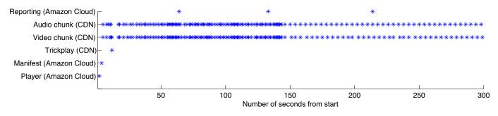
Fig. 2. Timeline in serving a Netflix client
