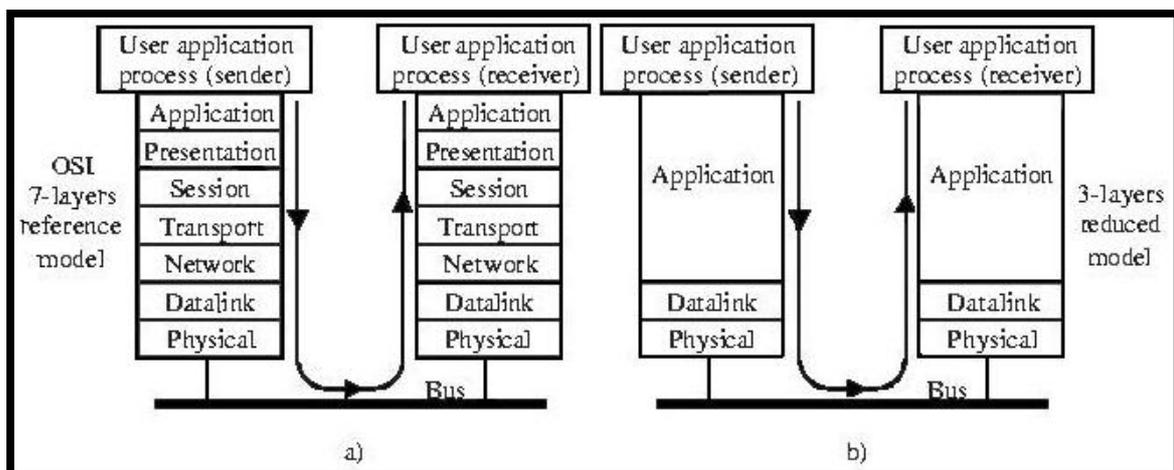
**Fig. 1.8.** The OSI 7-layers reference model (a), and the reduced fieldbus 3-layer structure (b).
