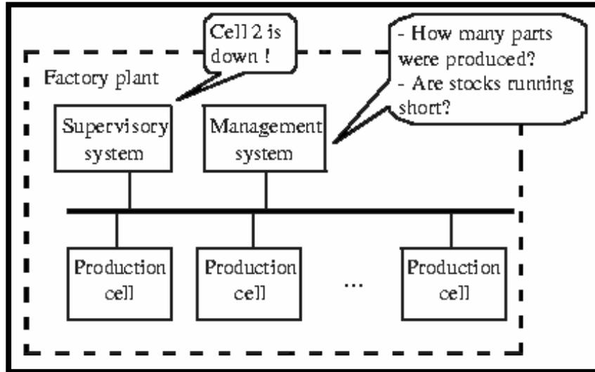
**Fig. 1.5.** The trend towards the use of a distributed architecture in manufacturing industry to interconnect cells across the plant.
