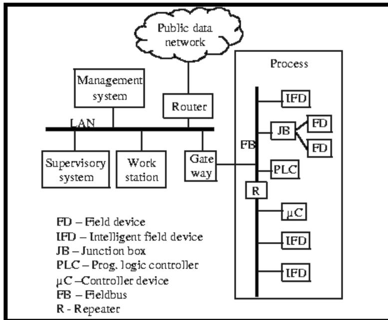
**Fig. 1.4.** The fully distributed architecture, based on a fieldbus, found in modern industrial automation systems.
