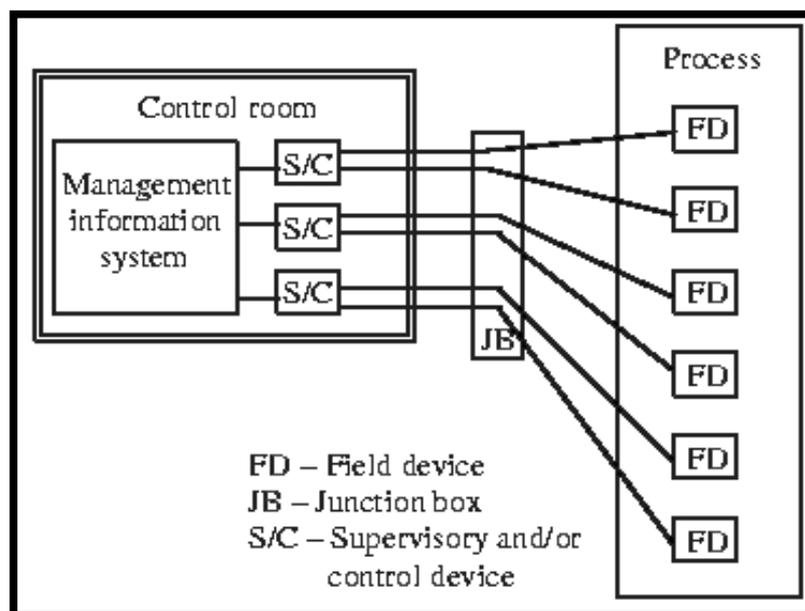
**Fig. 1.2.** The hierarchical architecture which was popular in Process Control Systems during the early 1970s.
