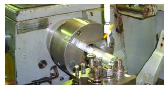
Figure 2. Arrangement for MQL for a feed rate of 0.5 mm/rev
