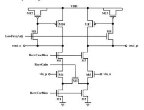
Figure 5 Schematic of the single stage preamplifier used by Fuller *et al.* The gain can be adjusted between 30 dB and 85 dB by adjusting RecvGain (1)
