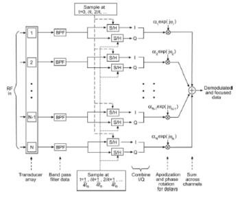
Figure 7 Diagram of the Direct Sampled I/Q Beamforming Algorithm (13)
