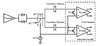
Figure 8 Diagram of the transmit protection circuitry as described by *Fuller et al.* (14)
