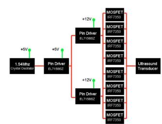
Figure 3 Block Diagram of the circuitry used be Lewis *et al.* to provide low output impedance (8)
