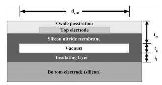
Figure 2 Diagram of a CMUT (from Oralkan et al.) (6)
