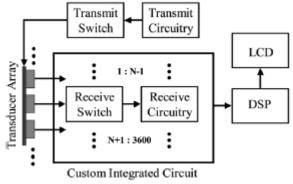
Figure 4 Block Diagram of the Sonic Window by Fuller *et al.* (1)
