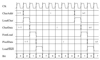
Fig. 4. A detailed timing diagram for the text-mode video controller. I teach the students such timing diagrams are crucial for designing functioning digital hardware.
