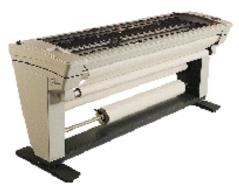
(C) Cutter Plotter for stencil design
