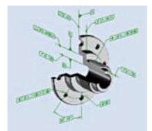
(F) Geometric tolerances on a solid model.
