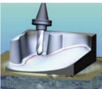
(E) Multi axis and multi spindle milling
