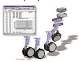
(D) Kinematics Analysis of landing gear
