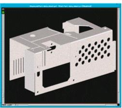
(B) A solid model of a sheet metal part
