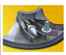
(F) Multi axis and multi spindle milling
