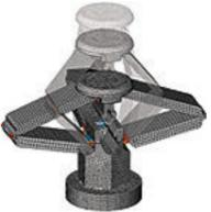
(E) Kinematics Analysis of support mechanism
