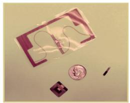
Fig. 2.1 Three different RFID tags they come in all shapes and sizes.
