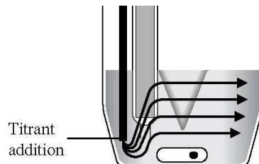
If a longer stirring bar is used, turbulence is not achieved and the mixing effectiveness is lower. Iodine would not be distributed upwards, but rather along the base directly towards the sensor.
