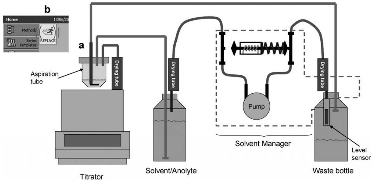
Step 1a: Put the draining and reagent refill tube into the coulometric titration cell.
