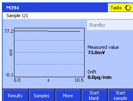
The weight of the solvent (msol), the weight of the sample (mext) and the weight of the aliquot of the supernatant solution containing the extracted water (sample size m) is entered into the respective sample data fields:
