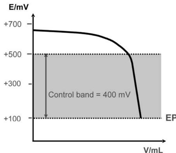
The titrant addition is calculated on one hand by using the distance of the actual potential from the end point and on the other by using  $dE/dt$ . The closer the potential to the end point, the slower is the titrant addition. Thus, if the control band width is decreased, the control reacts more sensitively to potential changes, which leads to a stronger reduction of the dosing speed. The dynamics of the control can be influenced in the following way:
