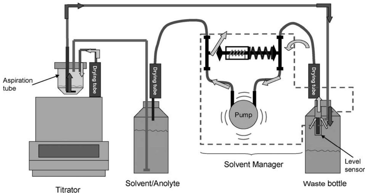
Step 2: The Anolyte is drained into the waste bottle by applying vacuum.
