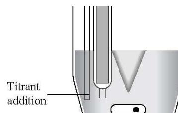
bubbles form into the solution, the stirring speed is too fast. Bubbles falsify the measured values.
