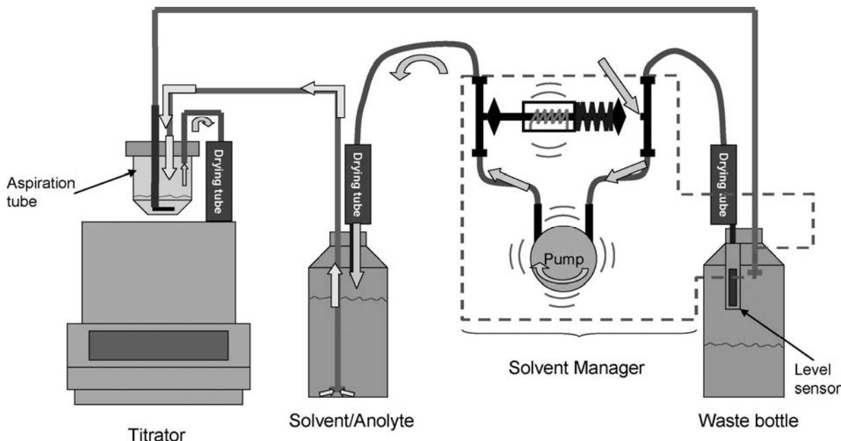
Step 3: The pump direction is switched by activation of the magnetic valve and subsequently fresh solvent is pumped into the titration cell by applying over pressure of dry air.
