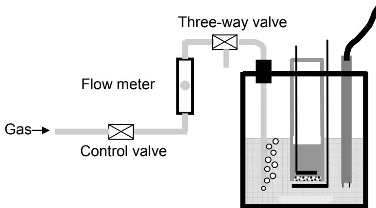
The flow rate has to be constant to determine the volume necessary to calculate the water content: gas volume = gas flow rate x time.
