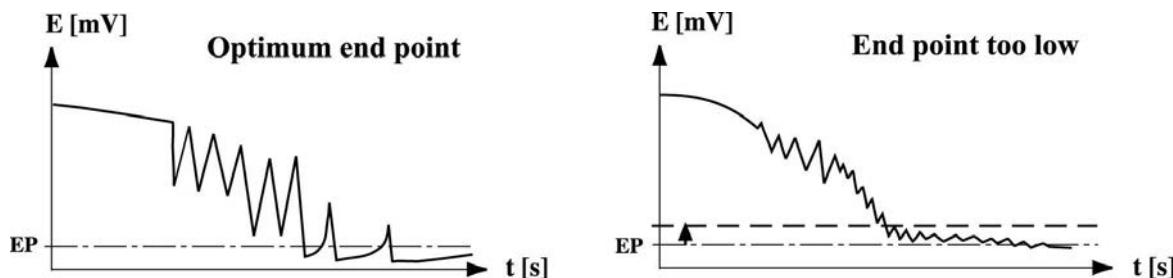
The consequences of choosing a too low end point value are illustrated in the figures above: On the right side, the titration curve is more or less flat towards the end; this results in an ill-defined titration end point, which will lead to long titration times and to low precision.
