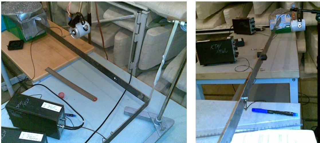
Figure 1: The test objects and their arrangement. To the left the right angled steel beam and to the right the straight steel beam with a magnet mass attached. The beams are embedded in sand boxes in the end to suppress reflections. The right angled beam is supported with a rubber band at the corner.
