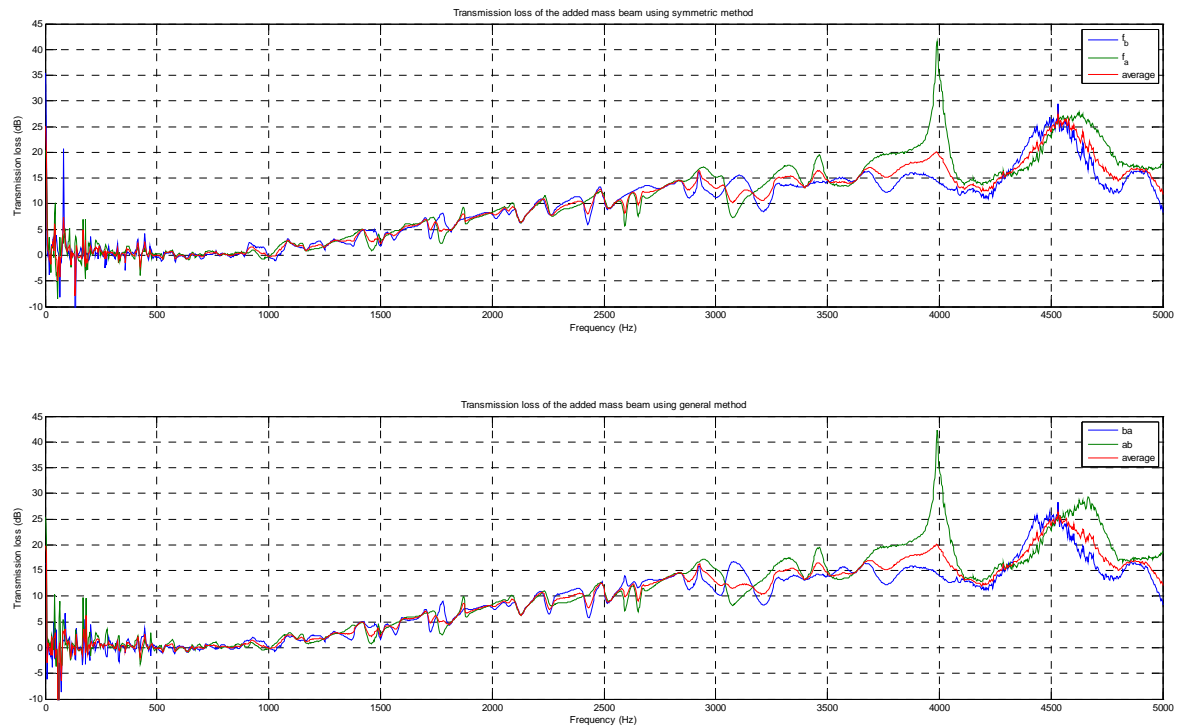
Figure 4b: Comparison of the two groups of measurements and its average of the measured structure-borne sound transmission loss when mass is added to the beam. The upper curve is showing the simplified method and the lower curve is showing the general method. Note the peak at 4 kHz when exciting point of beam A is being used.
