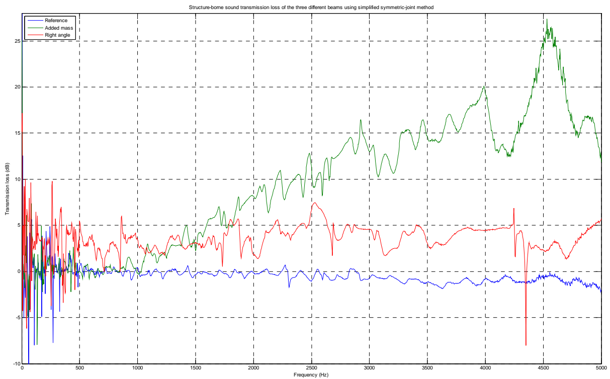
Figure 3: Comparison of the measured structure-borne sound transmission loss of the reference beam, the straight beam with added mass and the right angled beam. The average of the two groups of measurements is used with the simplified symmetric-joint method.
