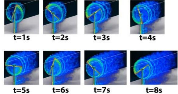
**Figure 6.** Single Turbine Results showing vortical structure around the turbine at varying times  $t=1, 2, 3, 4, 5, 6, 7, 8$  s, respectively. Inlet wind velocity was set to  $5\text{m/s}$  at hub height. The NREL Phase VI two-bladed turbine was used in the simulation
