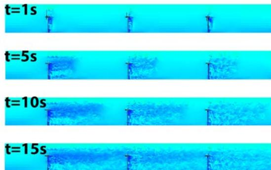
**Figure 9.** Three in-line turbine results showing instantaneous vortical structure around the turbine at varying times  $t=1, 5, 10, 15$  s, respectively. Inlet wind velocity was set to  $5\text{m/s}$  at hub height. The NREL Phase VI two-bladed turbines were used in the simulation. The vorticity magnitude contours are plotted with the use of identical scales
