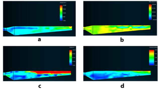
**Figure 7.** surface contours at  $10\text{s}$ . (a) velocity. (b) pressure. (c) vorticity. (d) turbulence intensity
