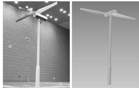
**Figure 2.** Unsteady aerodynamics experimental turbine in the NASA Ames 80 ft by 120 ft wind tunnel (left) and Model turbine used in current study (right)
