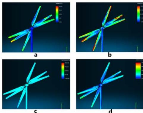
**Figure 10.** Surface contours of three in-line turbines (superposed) at  $14.84$  s. (a) velocity. (b) vorticity. (c) pressure. and (d) turbulence intensity
