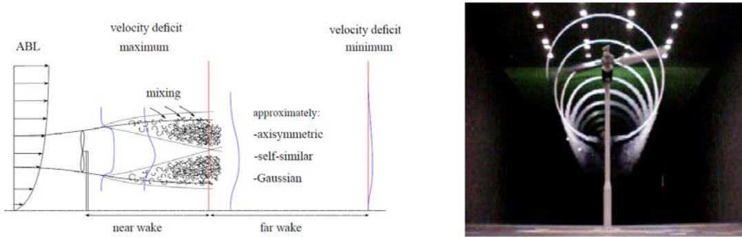
**Figure 1.** Aerodynamics of the wake of a wind turbine (left) and vortical wake visualization behind a horizontal axis wind turbine (right) in the wind tunnel at NASA Ames Research Center [4]
