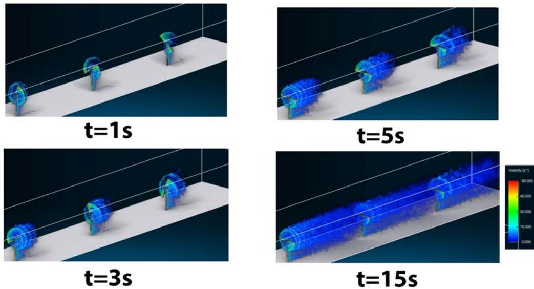
**Figure 8.** Wake Interaction among three inline turbines. Turbine Results showing vortical structure around the turbine at varying times  $t=1, 3, 5, 15$  s, respectively. Inlet wind velocity was set to  $5\text{m/s}$  at hub height. The NREL Phase VI two-bladed turbine was used in the simulation
