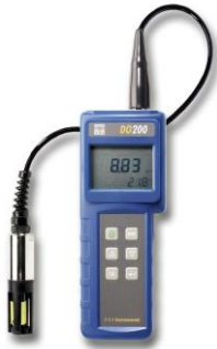
The EcoSense DO200 is available with a 4- or 10- meter cable.
