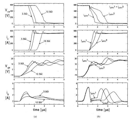
Fig. 7. Measured turn-on switching waveforms  $(v_{ce}, i_c, v_{ge}, i_g)$  with (a) the CGD and (b) the AGD when the turn-on di/dt is varied. Turn-on gate resistors used for varying di/dt in the CGD are 3.5, 5.6, and 12.5  $\Omega$ . Other conditions are as follows:  $V_{dc} = 600$  V;  $I_L = 500$  A;  $V_{gg+} = 18$  V;  $V_{gg-} = -12$  V.
