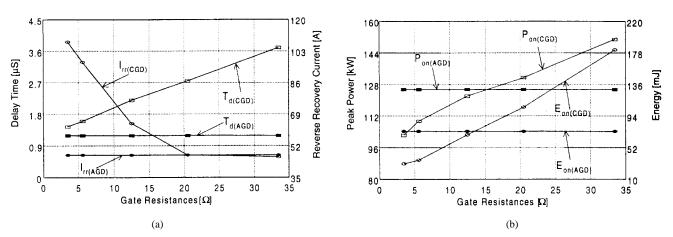
Fig. 8. Comparison of turn-on characteristics between the AGD and the CGD as gate resistance is varied. (a) Investigation of the turn-on delay time and the peak reverse-recovery current. (b) Investigation of the peak power and the turn-on energy loss. Operating conditions are as follows:  $V_{dc} = 600$  V;  $I_L = 350$  A;  $V_{gg+} = 18$  V;  $V_{gg-} = -12$  V.
