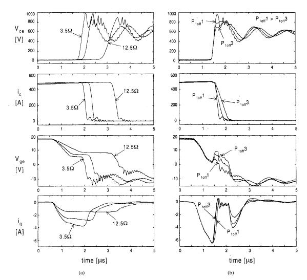
Fig. 10. Measured turn-off switching waveforms  $(v_{ce}, i_c, v_{ge}, i_g)$  with (a) the CGD and (b) the AGD when the turn-off di/dt is varied. Turn-off gate resistors used in the CGD for varying di/dt are 3.5, 5.6, and 12.5  $\Omega$ . Other conditions are as follows:  $V_{dc} = 600$  V;  $I_L = 500$  A;  $V_{gg+} = 18$  V;  $V_{gg-} = -12$  V.
