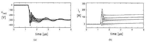
Fig. 6. Measured turn-on waveforms with the CGD at current levels of 0, 50, 80, and 120 A when the gate resistor of 0.5  $\Omega$  is used. (a) The freewheeling diode voltage. (b) The collector current. Other conditions are as follows:  $V_{dc} = 300$  V;  $V_{gg+} = 18$  V;  $V_{gg-} = -12$  V.
