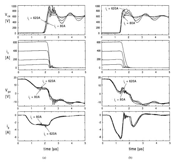
Fig. 9. Measured turn-off switching waveforms  $(v_{ce}, i_c, v_{ge}, i_g)$  with (a) the CGD and (b) the AGD at current levels of 80, 205, 405, and 620 A. Turn-off gate resistor used in the CGD is 5.6  $\Omega$ . Other conditions are as follows:  $V_{dc} = 600$  V;  $V_{gg+} = 18$  V;  $V_{gg-} = -12$  V.
