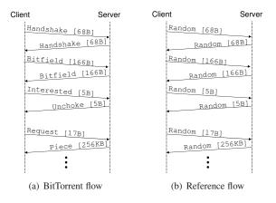
**Figure 3:** A pair of flows used in Glasnost tests. The two flows are identical in all aspects other than their packet payloads, which allows us to detect differentiation that targets flows based on their packet contents.
