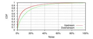
**Figure 5: Noise observed in our 3,705 sample dataset.** 85.2% of upstream flows and 75.7% of downstream flows have less than 20% of noise. Noise is measured as the difference between maximum and median throughput calculated as a percentage of maximum throughput.
