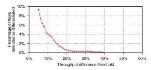
**Figure 6: Selecting a good throughput difference threshold.** Thresholds smaller than 20% tend to produce a significant number of false positives.
