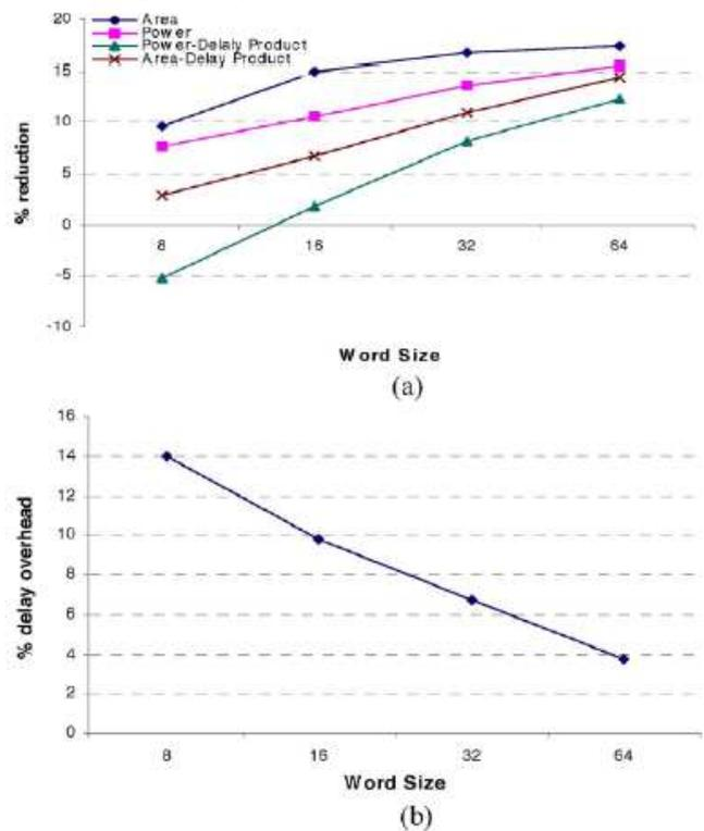
Fig. 8. (a) Percentage reduction in the cell area, total power, power–delay product, and area–delay product. (b) Percentage of delay overhead.
